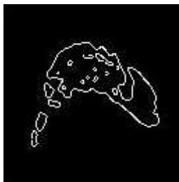
Fig. 4.12 Sobel edge detection on defective banana
