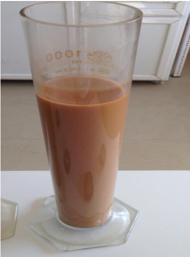
Figure 4.11: Sedimentation 1000 mL cylinder with distilled water and soil slurry
