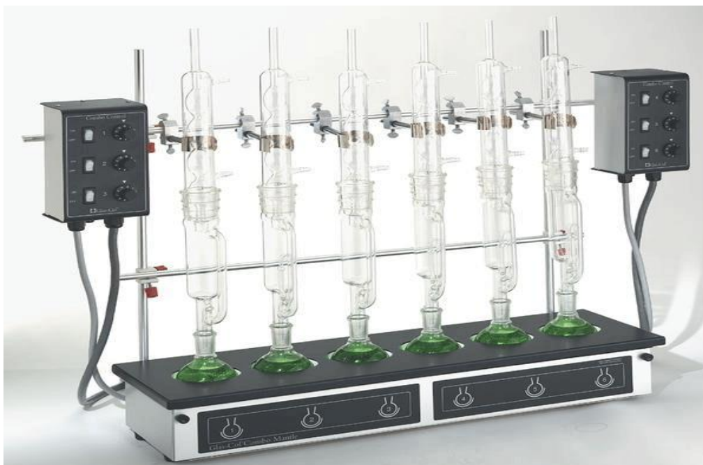
Figure 2.40: Reflux heating set up
