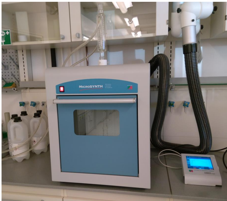
Figure 2.41: Microwave heating set up
