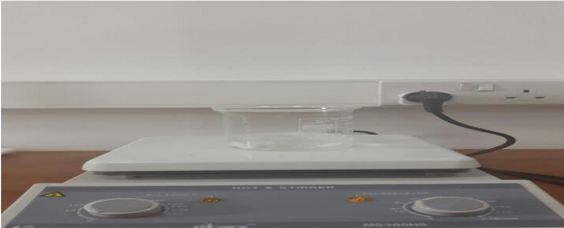
**Figure 2.5:** Prepared electrolyte solution of  $n\text{C}_2\text{H}_5\text{OH}:n\text{H}_2\text{O}:n\text{CaCl}_2$  at  $75^\circ\text{C}$
