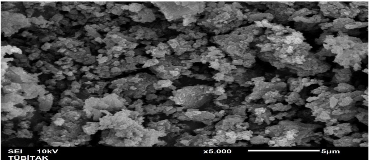
**Figure 3.11(d):** SEM of SF+0.20ml DEGDMA+0.05g of clopidogrel at x5000
