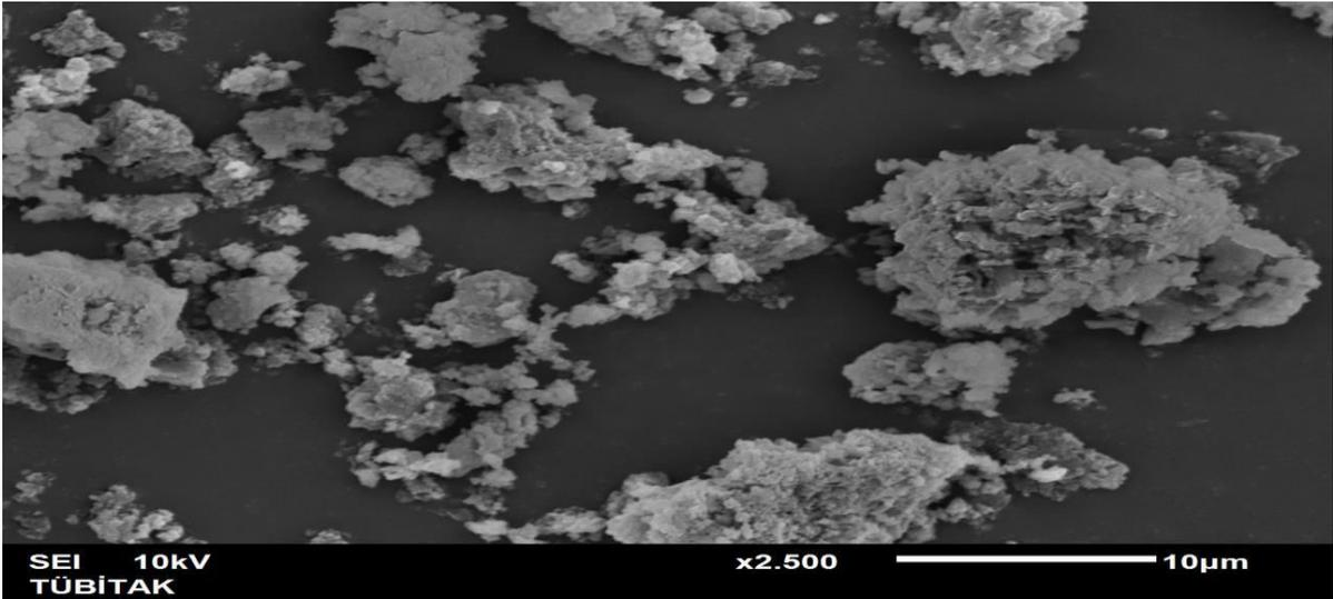
**Figure 3.11(c):** SEM of SF+0.20ml DEGDMA+0.05g of clopidogrel at x2500
