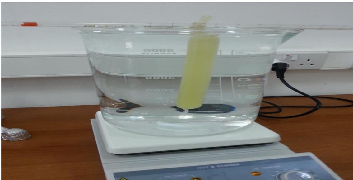
**Figure 2.7:** Aqueous silk fibroin electrolyte solution in tubing cellulose membrane tube
