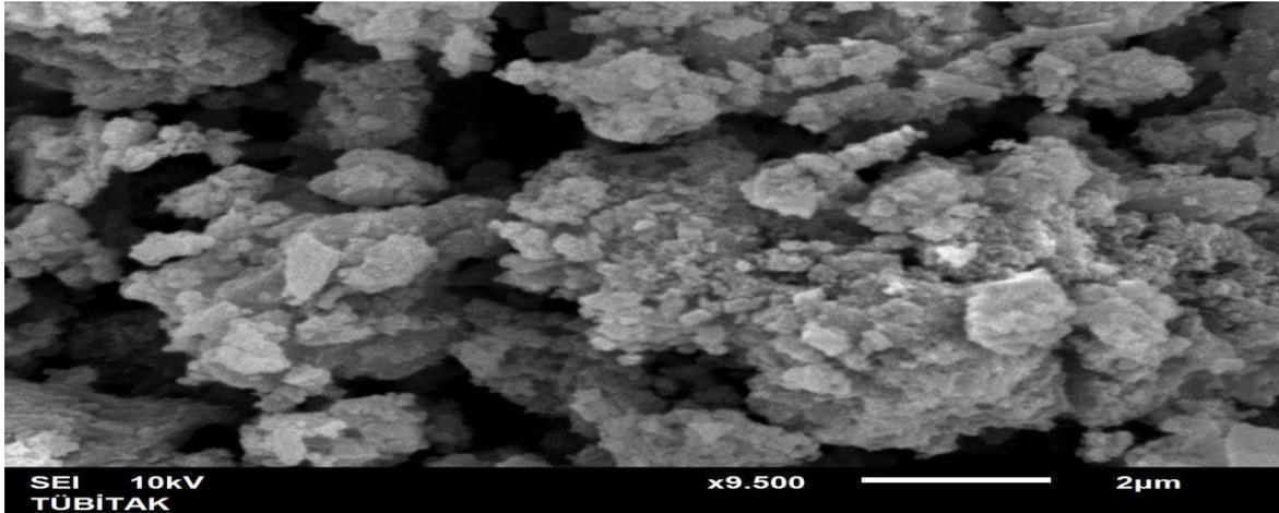
**Figure 3.11(e):** SEM of SF+0.20ml DEGDMA+0.05g of clopidogrel at x9500
