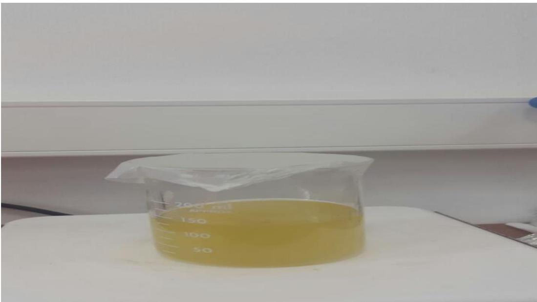
**Figure 2.6:** Dissolved 6% silk fibers in the electrolyte solution
