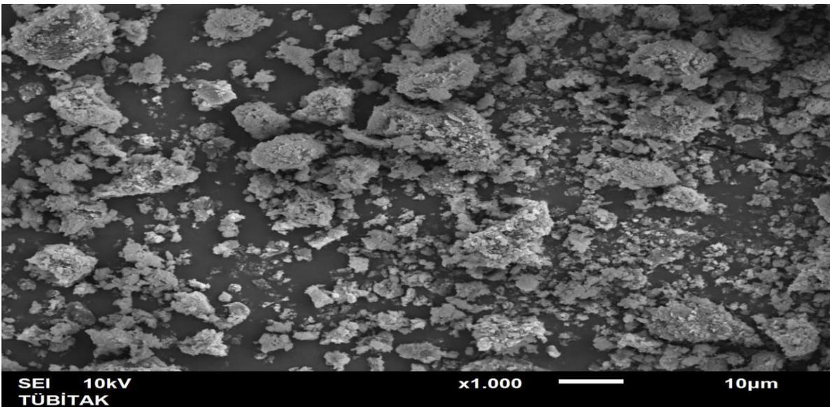
**Figure 3.11(b):** SEM of SF+0.20ml DEGDMA+0.05g of clopidogrel at x1000
