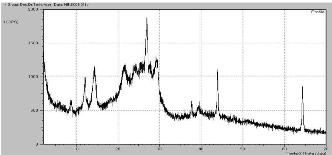
**Figure 3.13:** XRD analysis of Silk fibroin+0.20ml DEGDMA+0.05g clopidogrel
