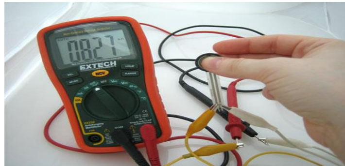
Figure 9: Testing the FSR
