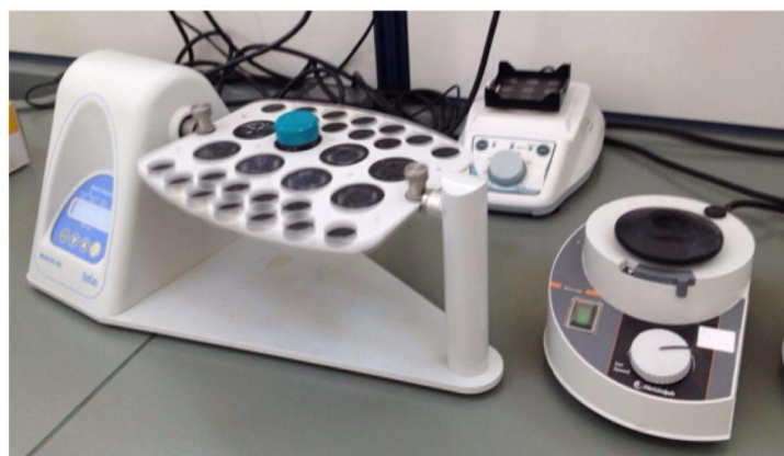
Figure 4.2c: Shaking of the extraction tubes with acetonitrile
