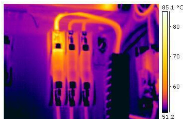
Figure 2.15: This thermo gram shows a fault with an industrial electrical fuse block (Huang, Yang & Tang, 1979)
