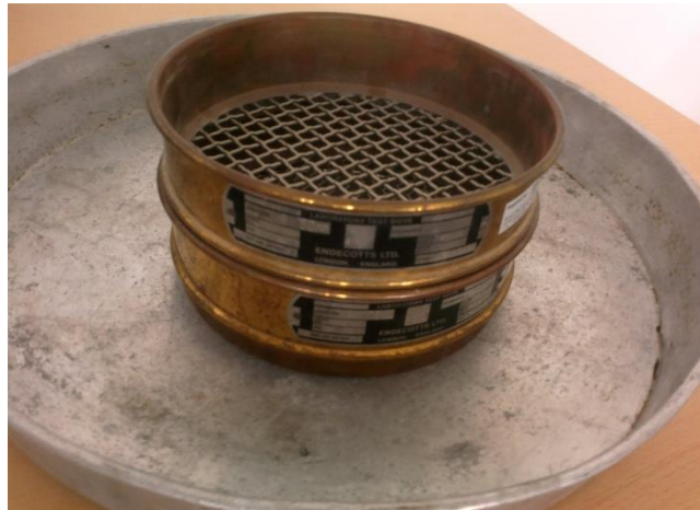
Figure 22: Two sieve of 0-4.75 and 5- 9.75 mm (Salimi, 2015)
