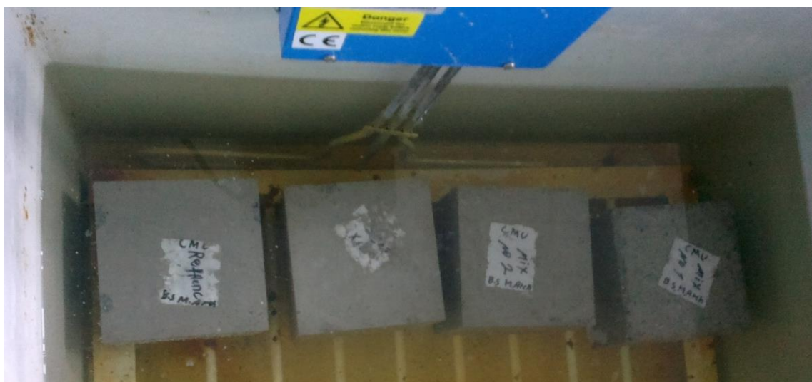
Figure 36: Specimens located in curing for 28 days (Salimi, 2015)
