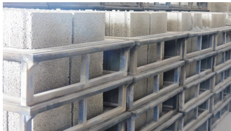
Figure 18: Produced CMU in rack (Salimi, 2014)
