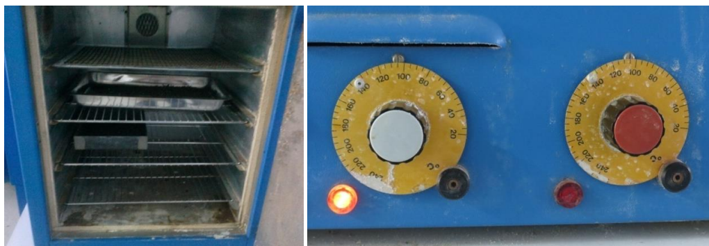
Figure30: Preparing oven for 24 hours in 105 °C (Salimi, 2015)
