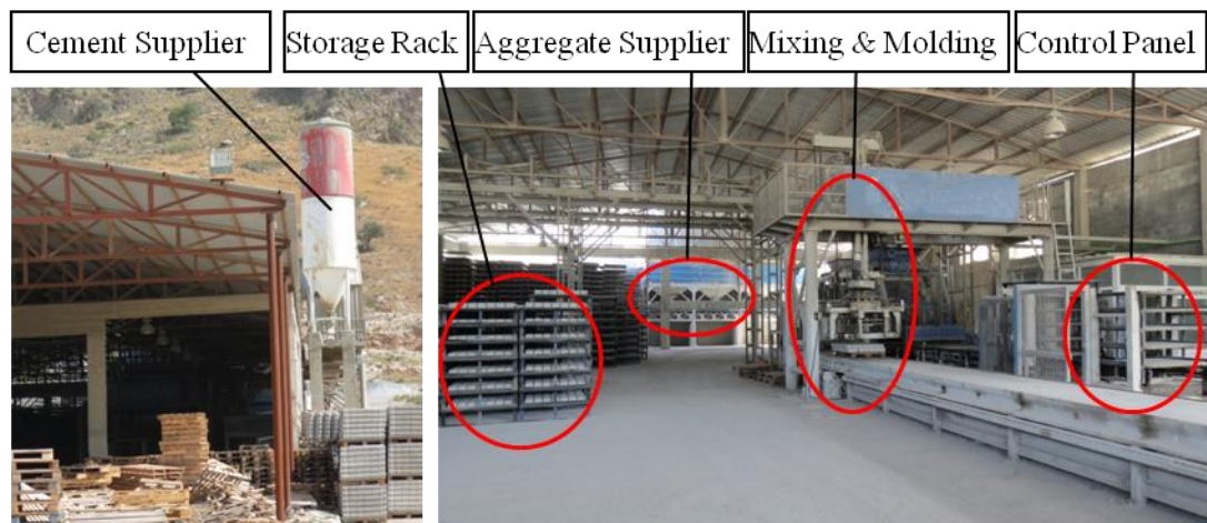
Figure 17: Precast concrete central plant, Nicosia (Salimi, 2014)
