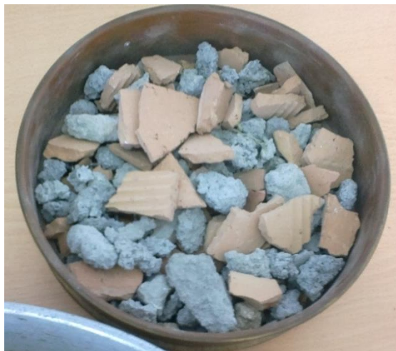
Figure 25: Remained larger parts of RA after sieve application (Salimi, 2015)
