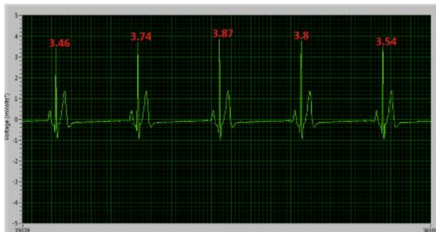
Figure 6.6: ECG Signal at 102.4 Hz Frequency
