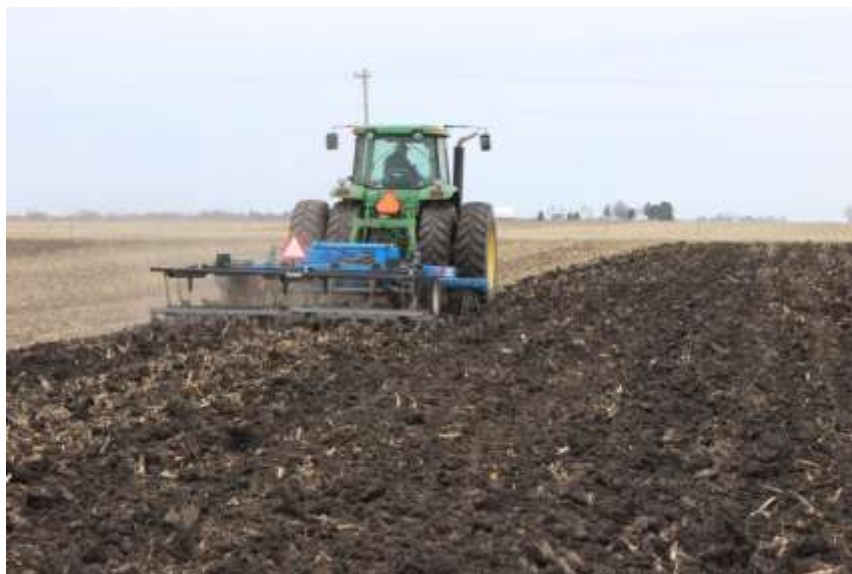
Figure 2. 2: A field that is being tilled by using a chisel plow. From “CONSIDERING CARBON NEUTRAL: TILLAGE OPTIONS,” by Troy (America’s Farmers, America’s Farmers, n.d.; Web; 1 Dec. 2016).
