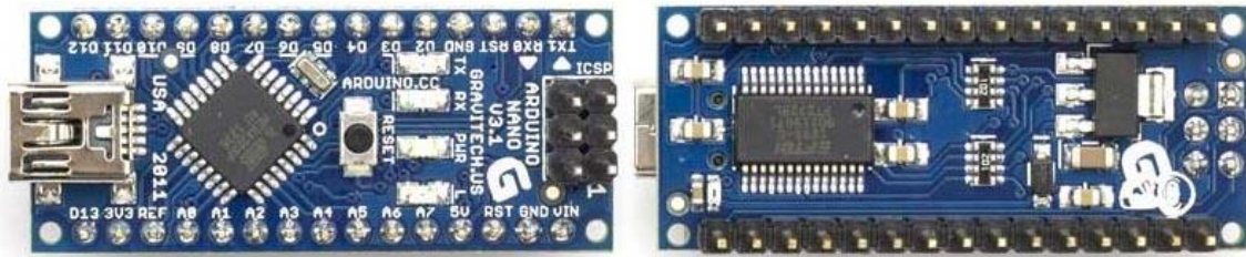
Figure 3.5: View of the front and back of the Arduino Nano card
