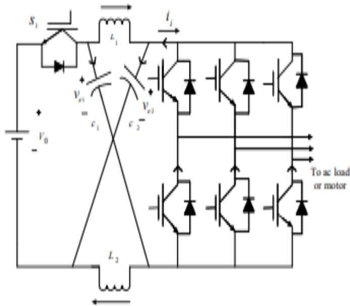
**Figure 2.2:** Bi-directional z-source inverter (Peng, F.Z.2003)
