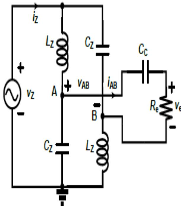
**Figure. 2.6:** A simple CPT circuit diagram showing Z impedance network
