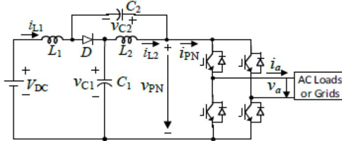
**Figure 4.1:** Proposed Circuit Diagram for simple phase QZSI
