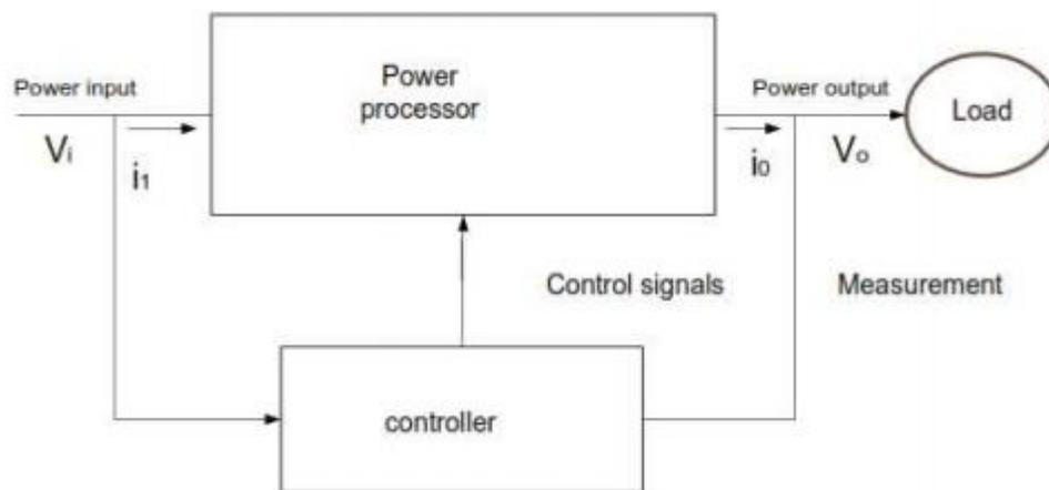
**Figure 2.15:** A power electronic system (Ja'far 2012)
