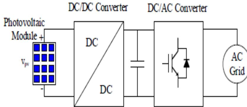
**Figure: 2.17:** 2 state GT- PV system arrangement
