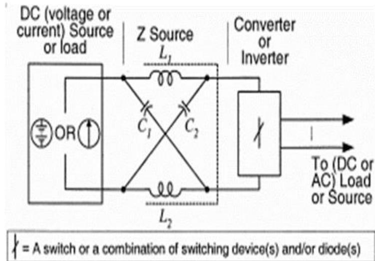
**Figure 2.1:** General structure of an Impedance-source converter
