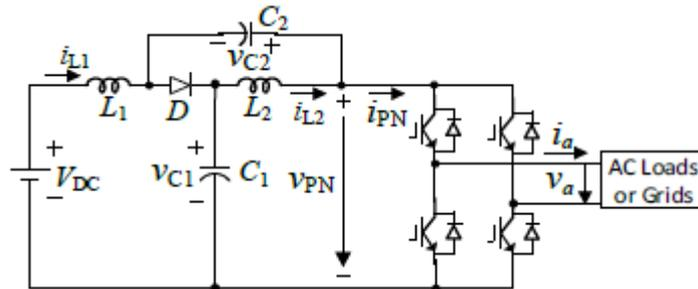
**Figure 3.1:** Schematic diagram of the proposed topology of S-P QZSI showing the direction of V and I
