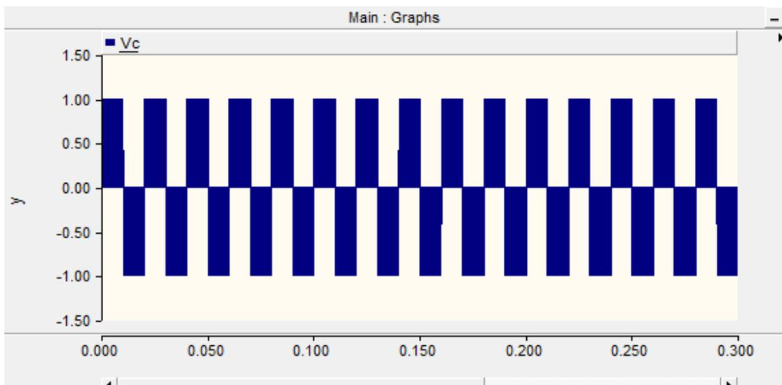
**Figure 4.10:** Voltage across capacitor
