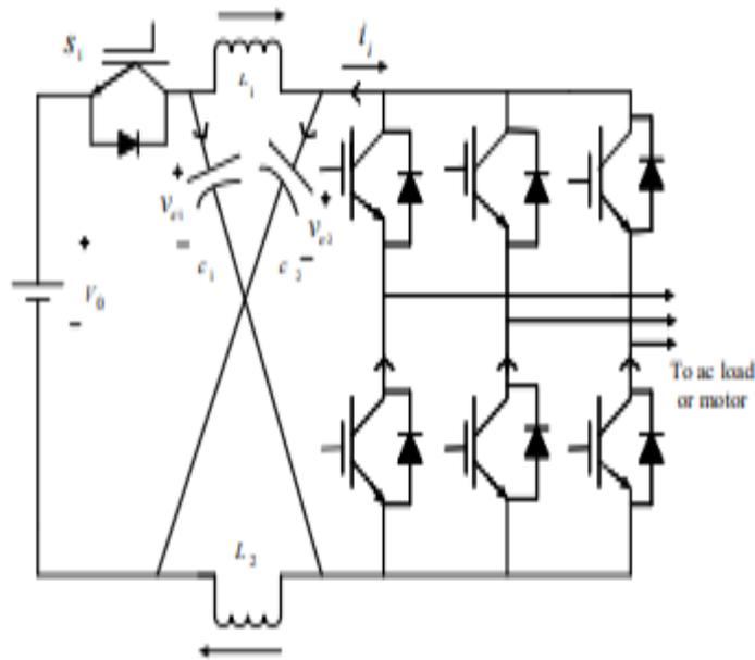
**Figure 2.2:** Bi-directional z-source inverter (Peng, F.Z.2003)
