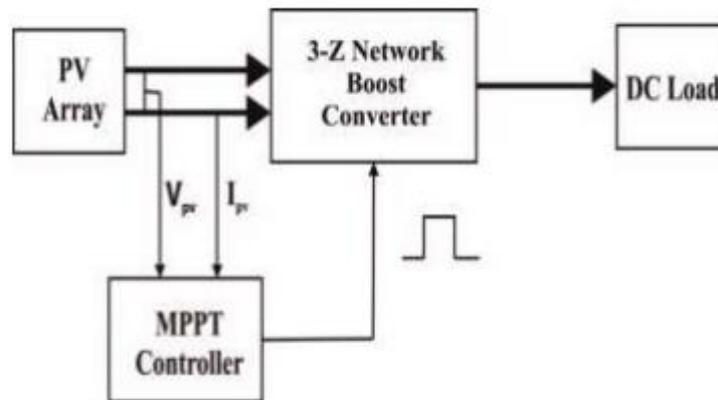
**Figure 2.14:** A proposed 3-Z Network boost system (kayatri et ai.,2016)
