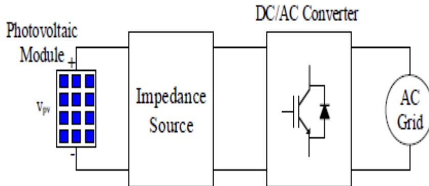
**Figure 2.18:** SPZ source GT-PV arrangement
