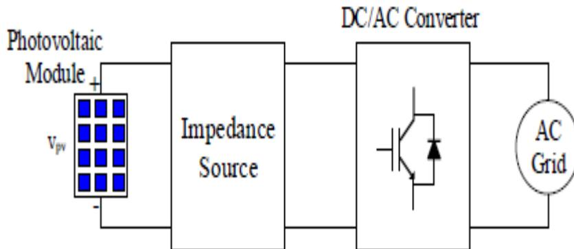
**Figure 2.18:** SPZ source GT-PV arrangement
