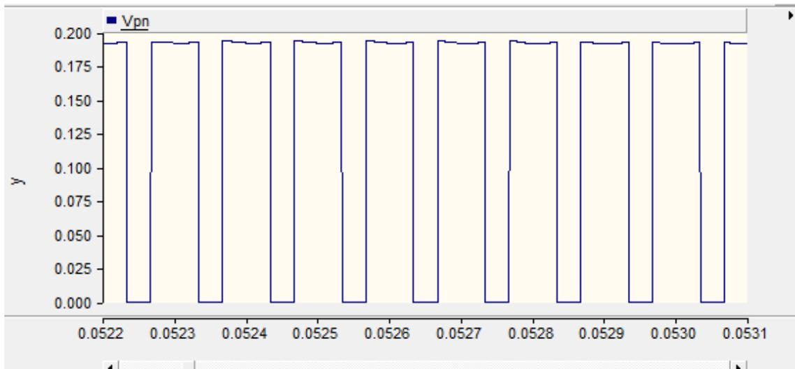
**Figure 4.7:** Average Direct current link peak Voltage envelope
