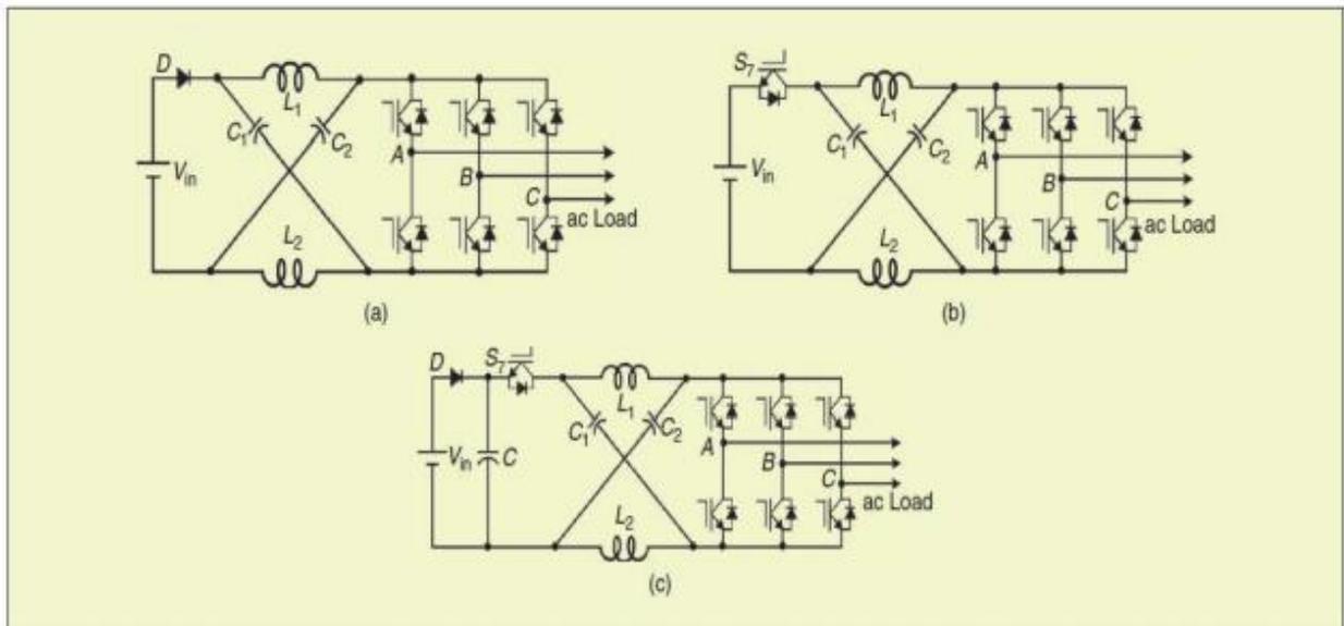
**Figure 2.3:** Impedance source inverter topologies a) ZSI b) Bidirectional ZSI (c) High performance ZSI (Peng, F. Z.; Ding. X.,2007)
