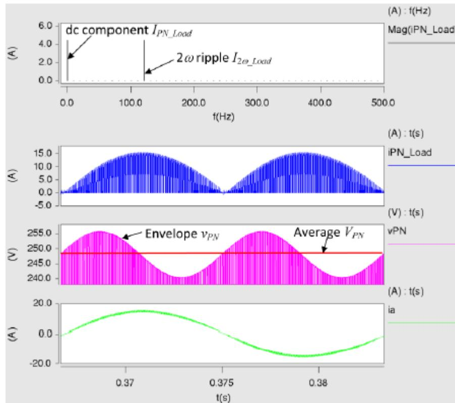
**Figure. 3.2:** Illustrating the double line frequency of the direct current link
