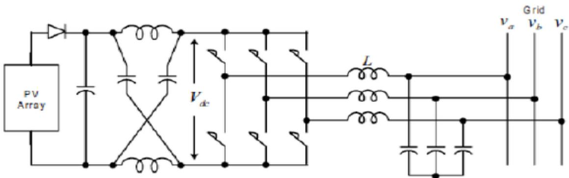
Figure 2.8: Three phase grid connected system
