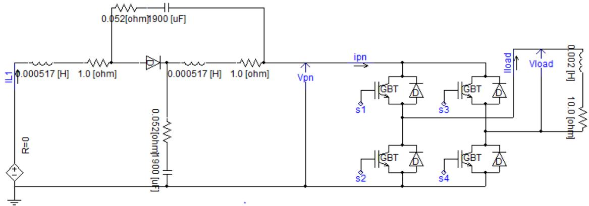
**Figure 4.2:** PSCAD Designed Circuit Diagram for Single phase QZSI
