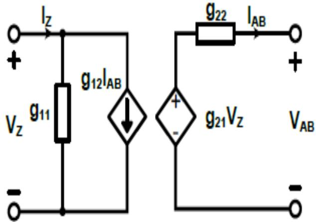
Figure. 2.7: The Z impedance network showing g-parameters
