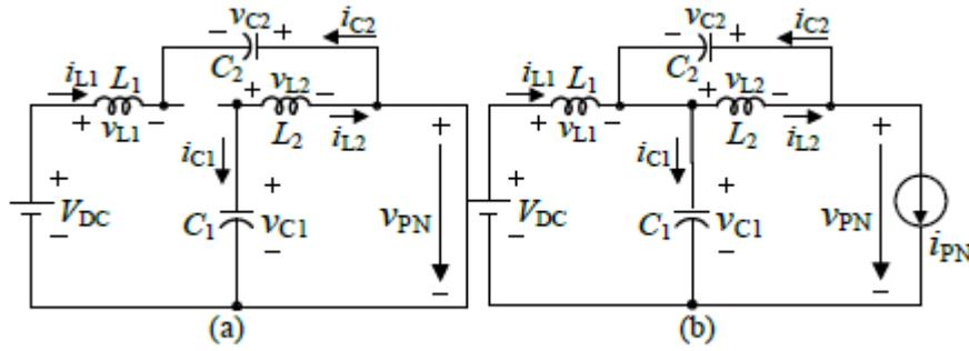
**Figure.3.3:** The S-P QZSI equivalent circuits. (a) shoot-through state; (b) non-shoot-through state
