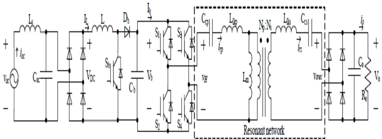
**Figure 2.12:** Step-up on-board battery charger
