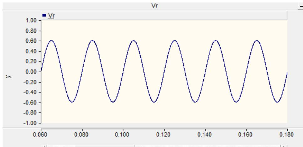
**Figure 4.3:** The Voltage of the load inductive resistance
