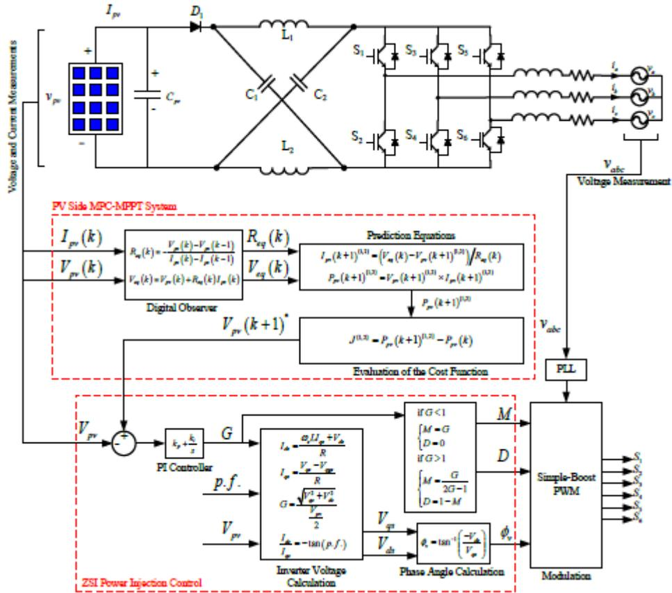
Figure: 2.19: The GTZSI and its regulated system
