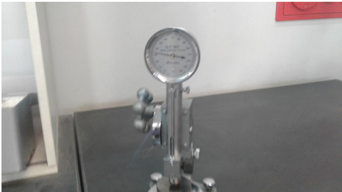
Figure 3.14: Shore hardness tester of Libyan Iron and Steel Company, Misurata Factory, Libya
