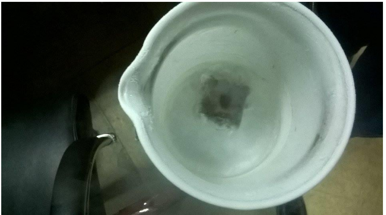
Figure 3.16: Nitrogen liquid bath for cooling the hardness specimens
