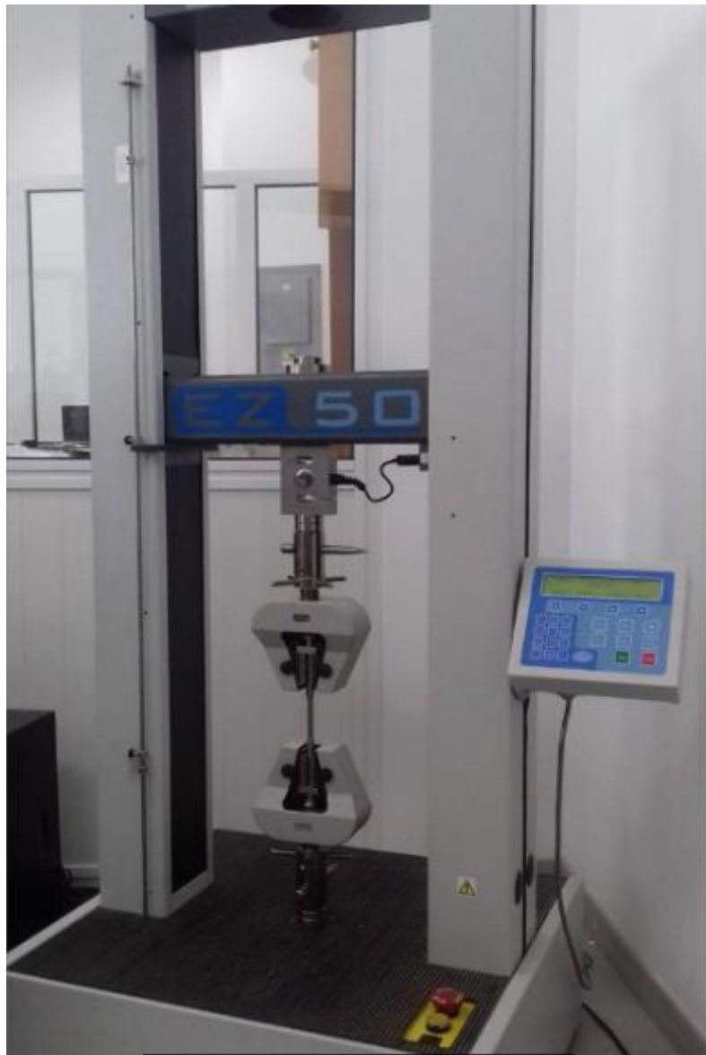
Figure 3.9: LLOYD EZ 50-universal tensile testing machine at the Mechanical Engineering Laboratory, NEU
