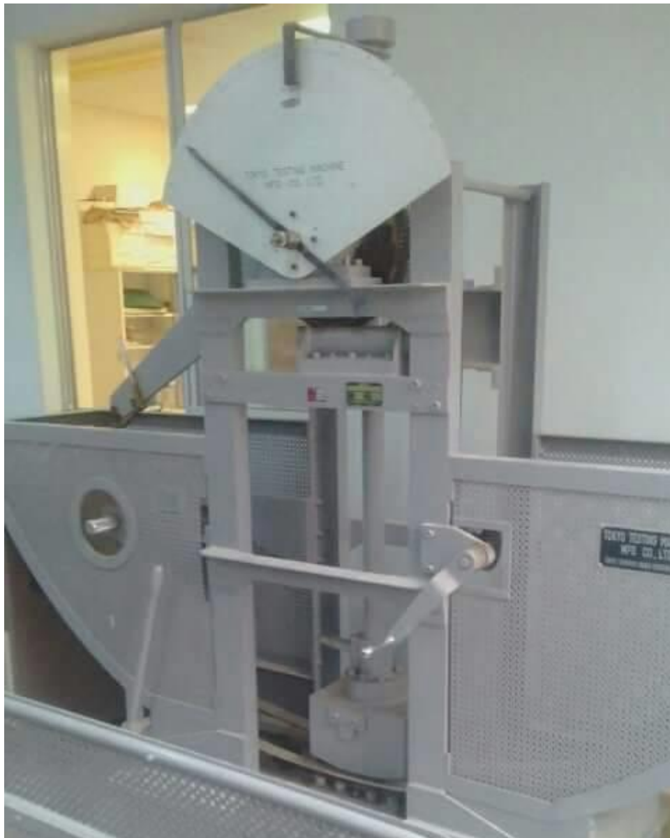
Figure 2.5: Impact Testing Machine (Izod) available in Libyan Iron and Steel Company, Misurata, Libya
