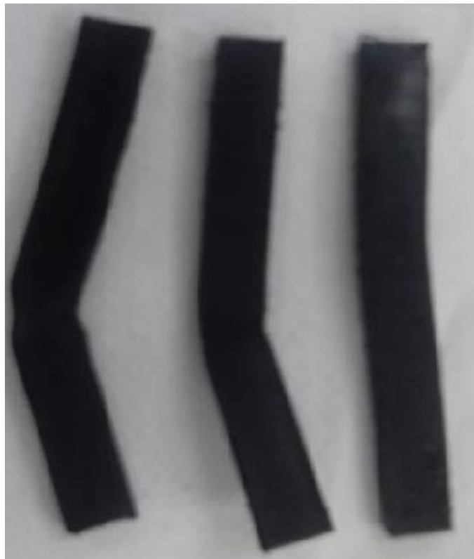
Figure 4.3: HDPE samples without notch after impact testing at RT carried out in Mechanical Engineering Laboratory, NEU (10mm (width)× 4mm (thickness)× 80mm (length))
