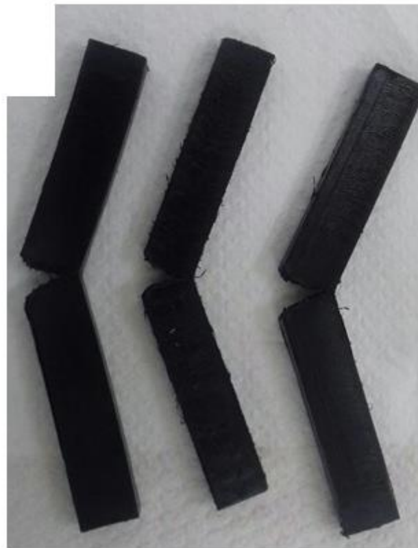
Figure 4.4: HDPE samples with notch after impact testing at RT carried out in Mechanical Engineering Laboratory, NEU) (10mm (width)× 4mm (thickness)× 80mm(length)) with 2mm depth (V)
