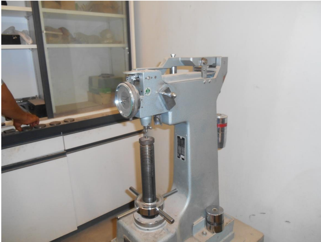
Figure 3.13: Rockwell Hardness tester (B) of the Libyan Iron and Steel Company, Misurata Factory, Libya
