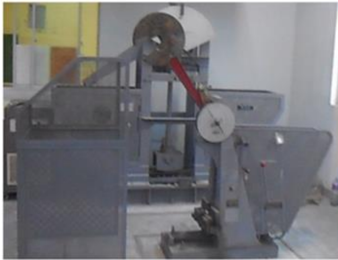
Tester for measuring the energy of API 5L X60 (Libyan Iron Steel works)
