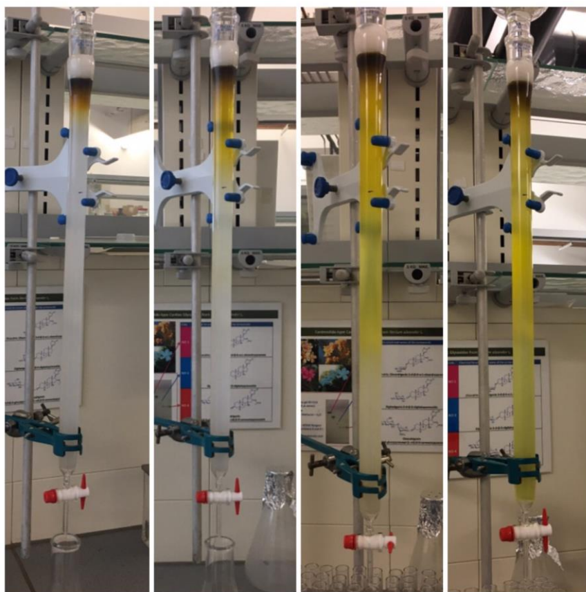
Figure 3.25: Isolation of piperine by column chromatography.
