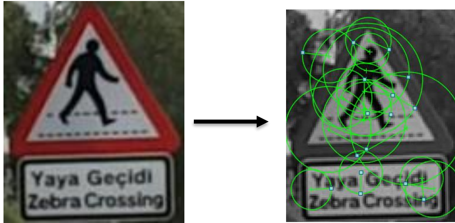
Figure 4.5: SURF key points detected in a traffic sign image.
