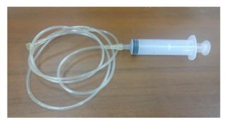
Figure 3.6: Suction instrument
