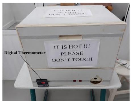
Figure 3.1: Constant temperature furnace controlled by digital thermometer
