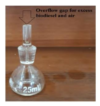
**Figure 3.9:** Overflow gap of pycnometer
