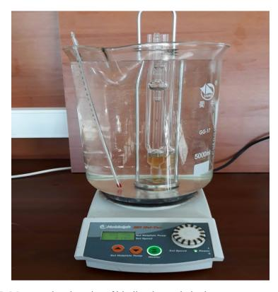
**Figure 3.5:** Measure the viscosity of biodiesel sample in the temperature range  $30^{\circ}\text{C}$  -  $90^{\circ}\text{C}$
