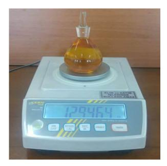
Figure 3.10: Pycnometer on the electronic scale
