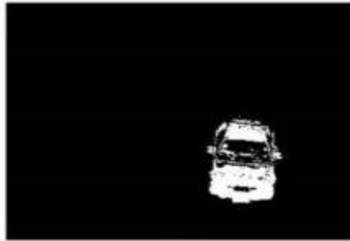
(c) The foreground image constructed by masked subtraction after shadow removal.
