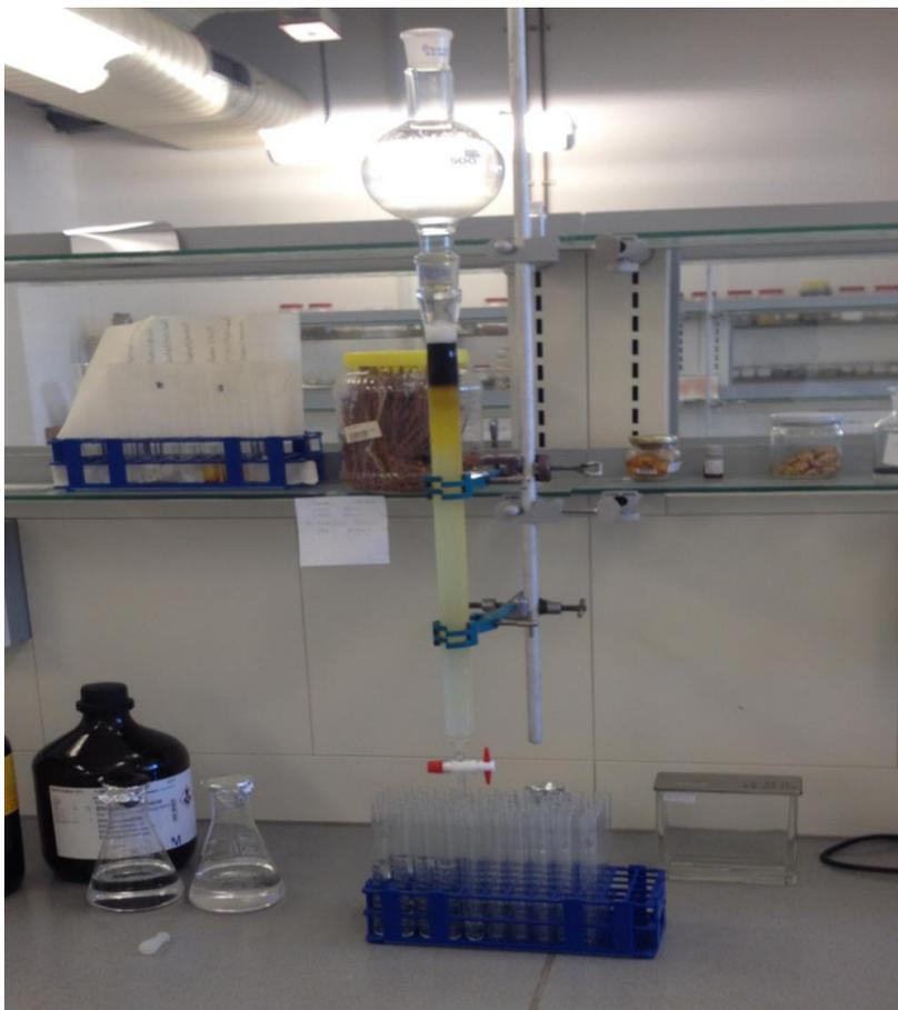
**Figure 3.34:** Setup of column chromatography containing the crude extract.
