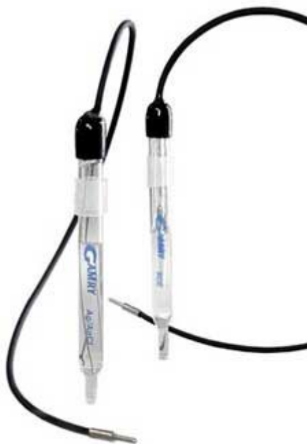
Figure 4.6: Reference electrode, i.e. Saturated Calomel Electrode (SCE)
