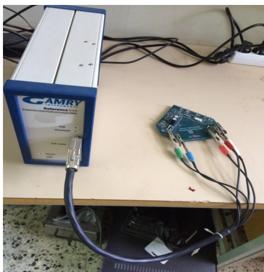
Figure 4.5: Calibration of the system with the dummy cell
