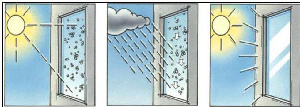
Figure 3.18: Diagram shows how photo catalysis work (Leydecker, 2008)
