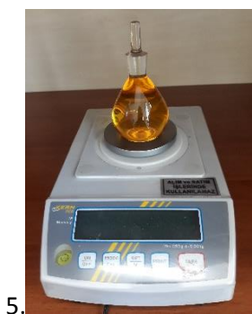
Figure 3.6: Diagrammatic representation of measuring density-using pycnometer
