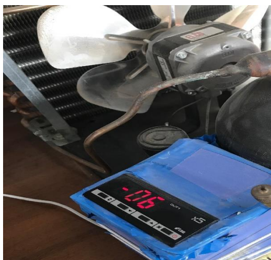
Figure 3.4: Thermostat attached to the cooling bath for measurements at low temperatures.
