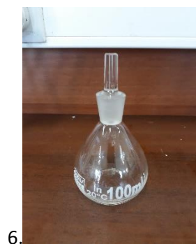
Figure 3.6: Diagrammatic representation of measuring density-using pycnometer
