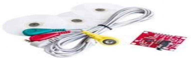
Figure 3.4: Electrodes of ECG sensor to attached
