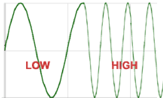
Fig 3.5: waveform showing low and high frequencies
