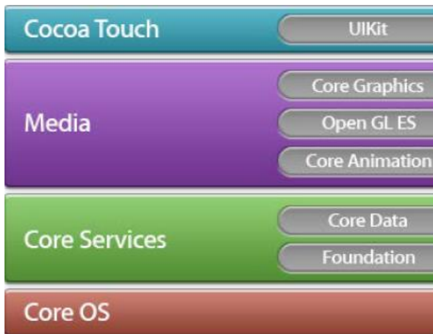
Figure 3.2: Architectural structure of the IOS operating system (Divya et al., 2016)
