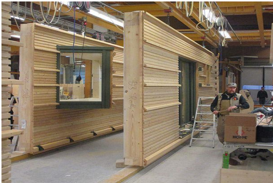
Fig. 3.30: Timber panel being manufactured in a factory (Brinkley, 2016)
