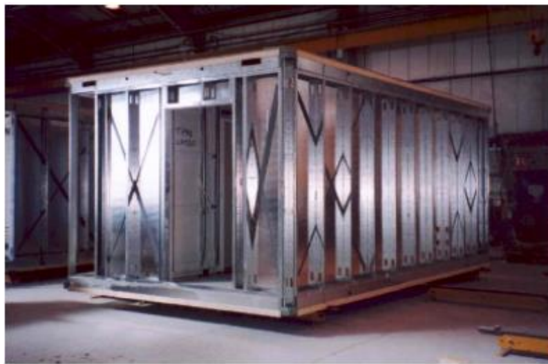
Figure 3.13: Typical 4-sided load-bearing module, (Steel Construction Info, n.d.)
