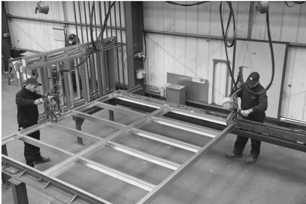
Figure 3.27: Manufacture of Light Steel Panel (Lawson et al., 2014)
