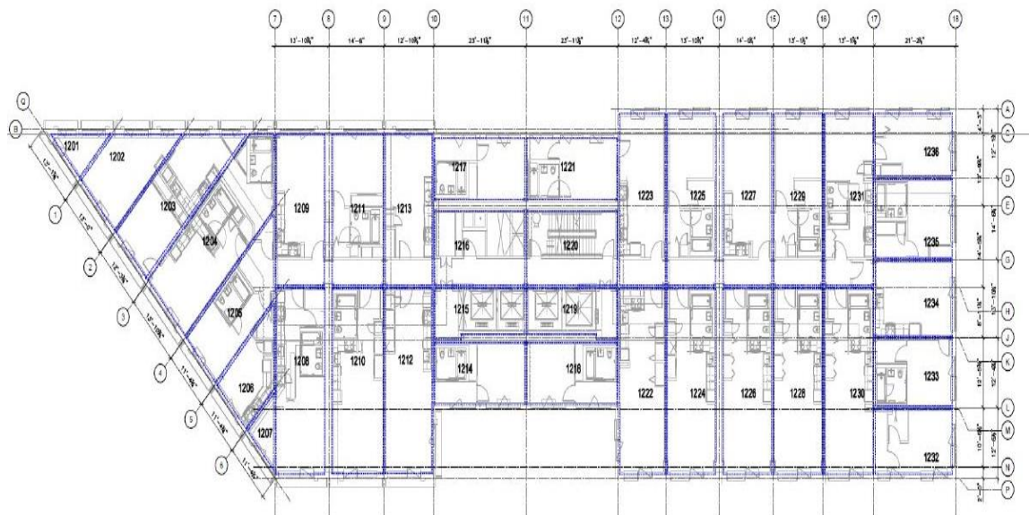
Figure 3.47: Typical floor layout of 461 Dean showing 36 modules per floor (Farnsworth, 2014)
