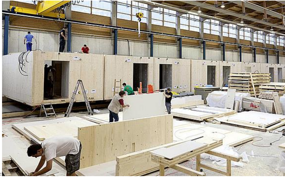
Figure 3.33: Factory fabrication of timber volumetric modules (Wölfl, 2016)
