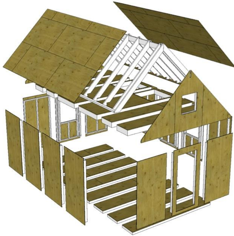
Figure 3.3: Constituents of a typical panelised construction (Janzen, 2011).
