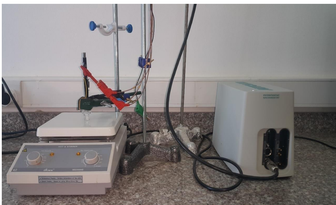
Figure 2.4: AutolabPotentiostat/Galvanostat connected to a 3-electrode electrochemical cell.
