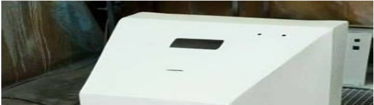
Figure 18.3: The body with the holes for Arduino components
