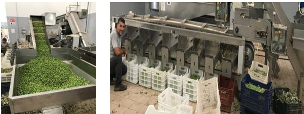
Figure 4.2: Separating olives from sorting machine
