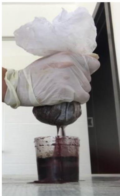
Figure 4.5: Filtering of fortified olive for salt analysis
