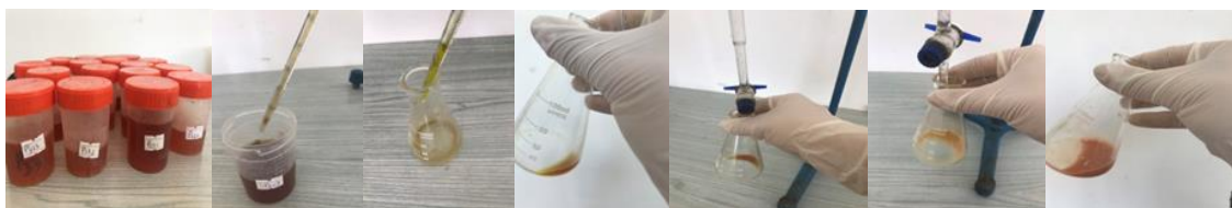
Figure 4.9: Salt analysis of olive's brine during the fermentation period
