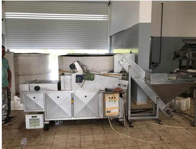
Figure 4.3: Craking olives in crushing machine
