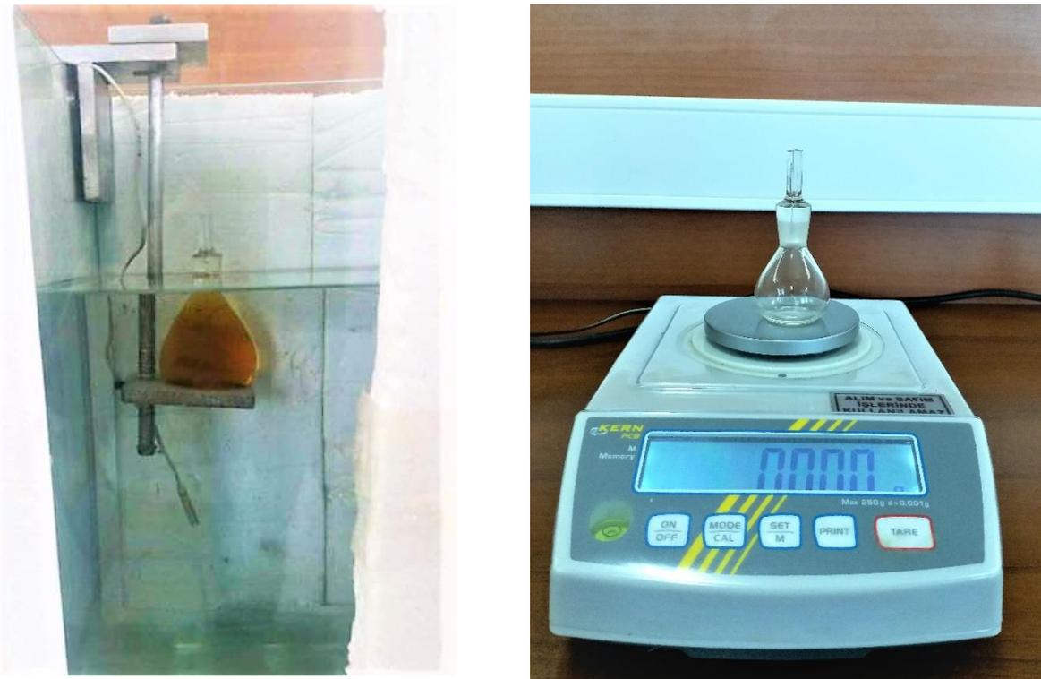
**Figure 3.13:** Setup of pycnometer in the cooling bath
