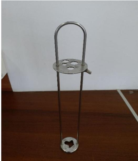
**Figure 3.6:** Viscometer holder
