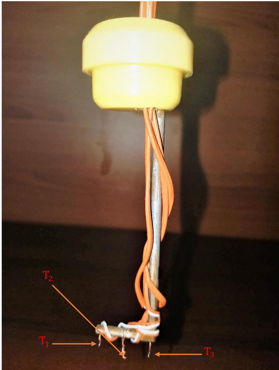
**Figure 3.17:** Thermocouple labelling for cooling curve
