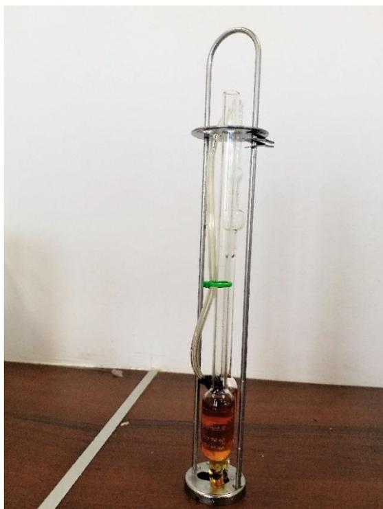
**Figure 3.10:** Ubbelohde Viscometer setup
