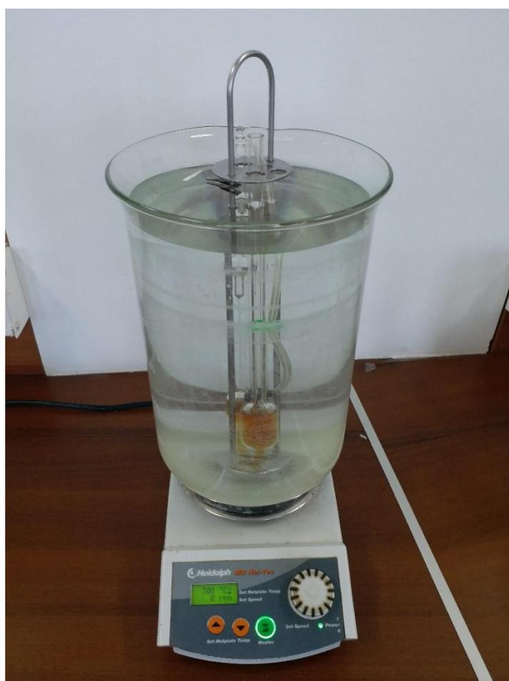
**Figure 3.9:** Experimental setup for kinematic viscosity measurement
