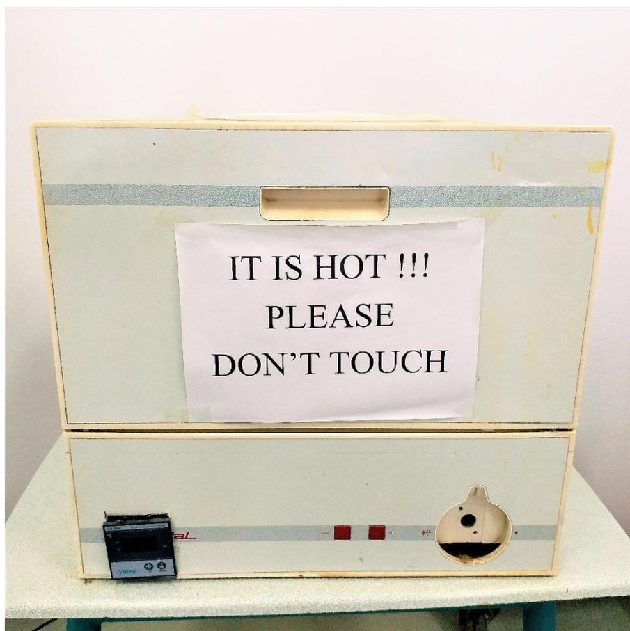
**Figure 3.3:** 40°C Temperature Controlled Oven
