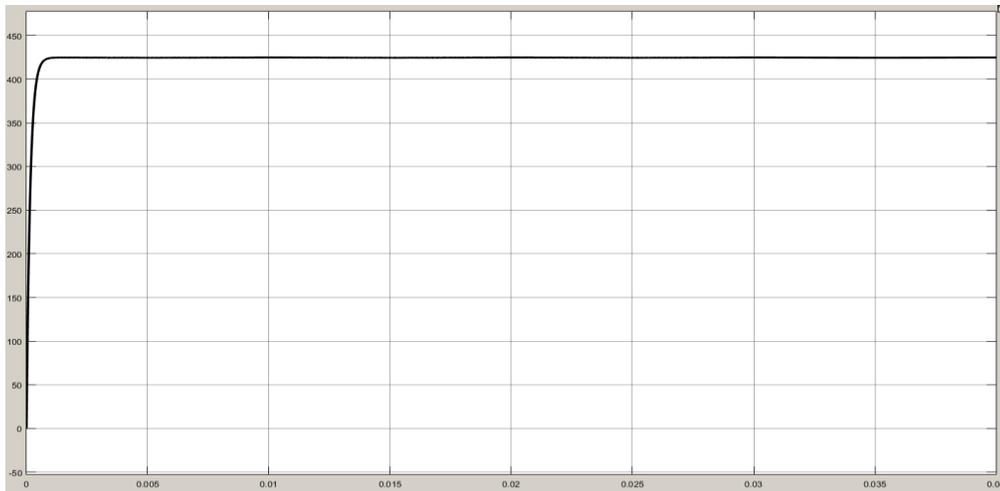
**Figure 5.3:** Boost converter output voltage waveform
