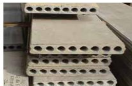
Precast concrete internal partition wall using copper slag
