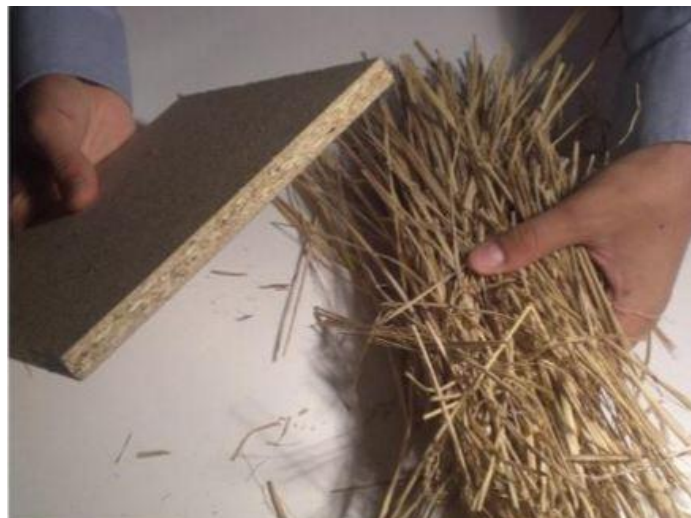
Figure 3.7: Rice straw as selected material for shelters (Elcharkawi, 2010)
