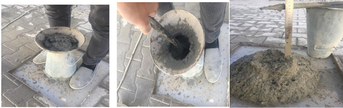
Figure 3.9: Stages of performing slump test
