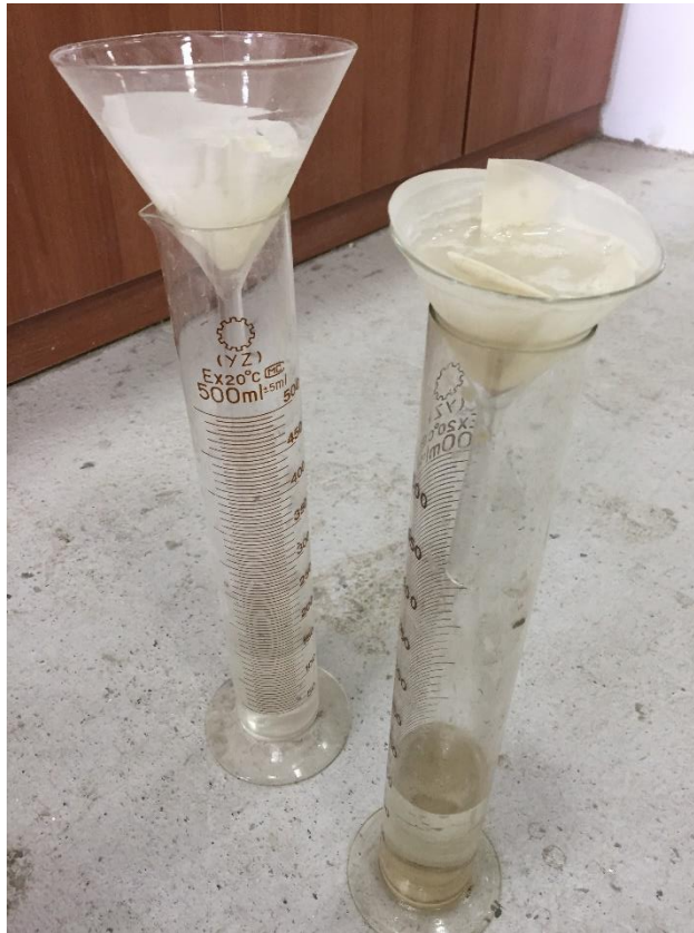
Figure 3.8: Extraction of water from fine aggregate by the help of filter paper.
