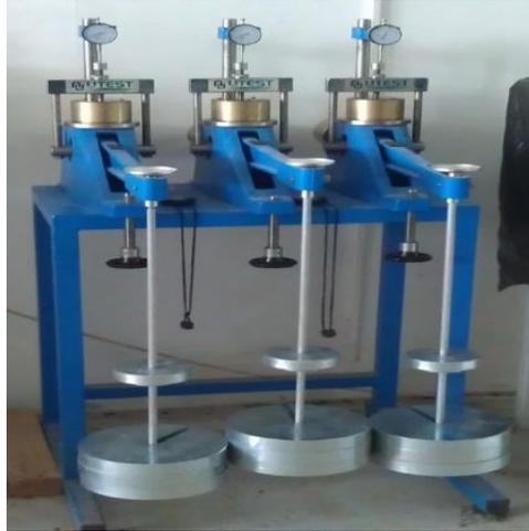
**Figure 3.6:** One-dimensional consolidation equipment
