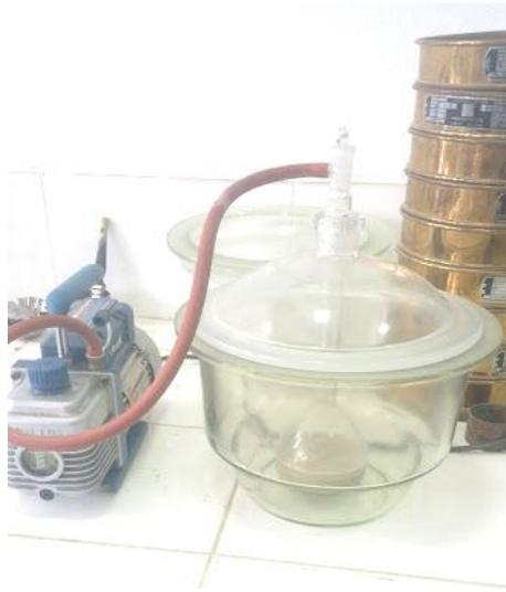
**Figure 3.2:** Vacuum pump and pycnometer
