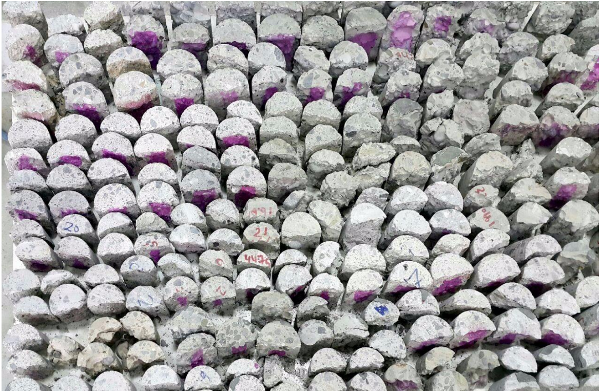
Figure 3.7: The samples after splitting and applying phenolphthalein, (NEU Civil Engineering Laboratory, 2018)
