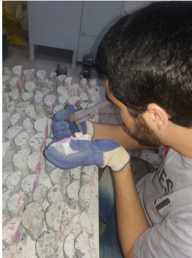
Figure 3.9: Measuring the carbonation depth by Vernier caliper, (NEU Civil Engineering Laboratory, 2018)
