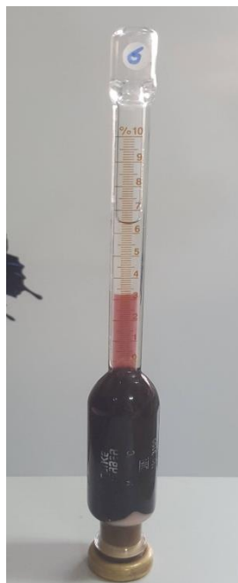
Figure 4.11: Sample prepared in the butyrometer for the analysis of milk fat ready to read after centrifugation
