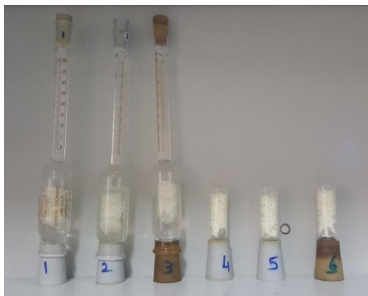
Figure 4.12: Butyrometer -prepared samples for cheese fat analysis
