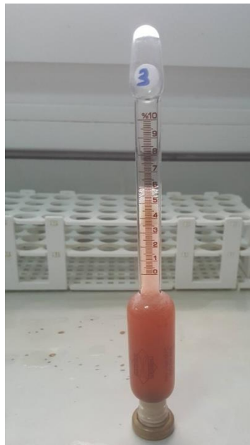
Figure 4.10: Mixture of samples prepared on the butyrometer for analysis of milk fat
