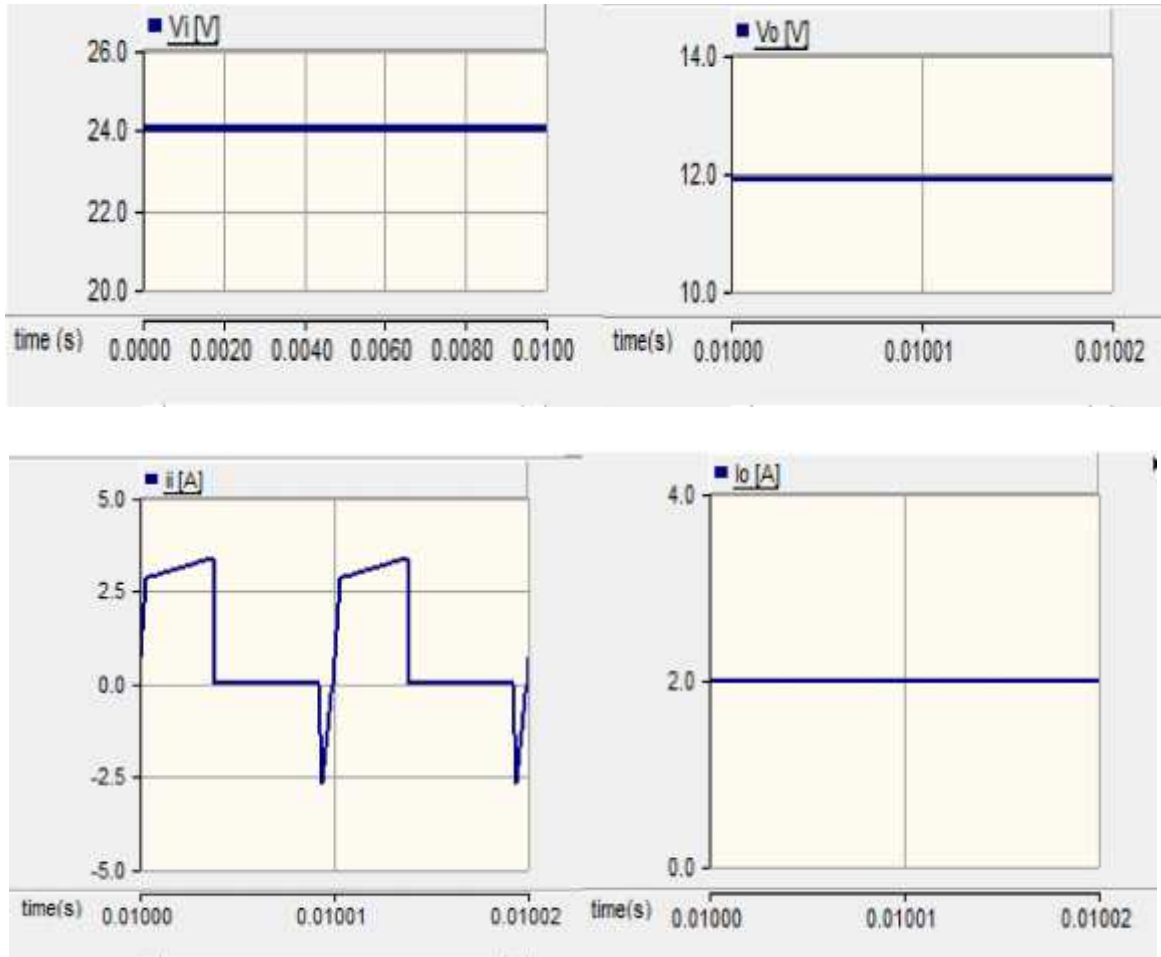
Figure 3.11: Input/output Currents and Voltage Waveforms
