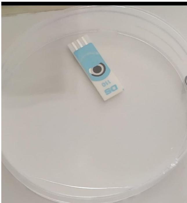
**Figure 3.3:** Screen printed electrode
