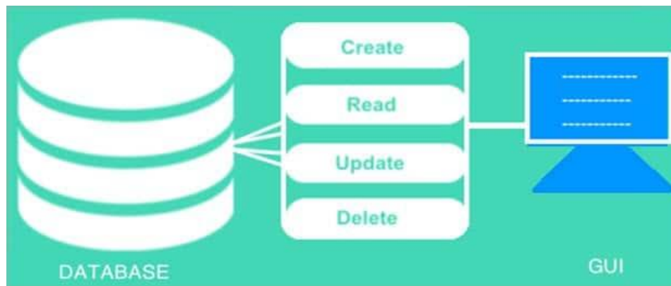
Figure 3.3: Show an overview of CRUD operations (Software Testing Help, 2019)
