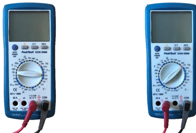
Figure 4.5: Multimeter used for measurement the current and voltage
