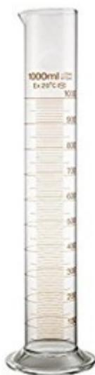
**Figure 3.2:** Measuring Cylinder
