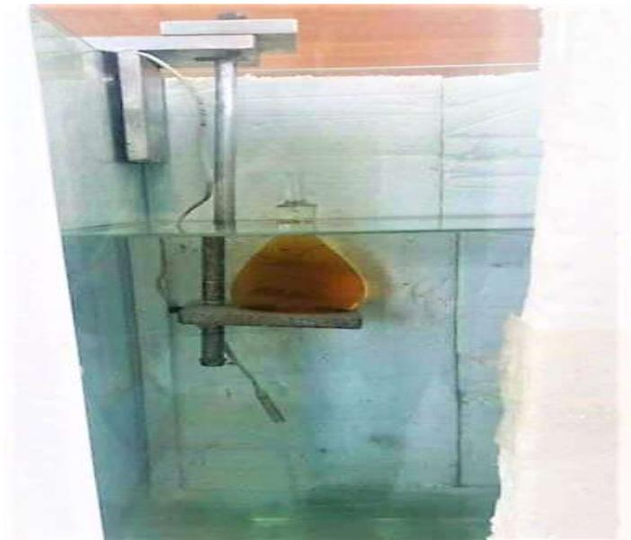
**Figure 3.9:** Setup assembly of cooling bath and pycnometer
