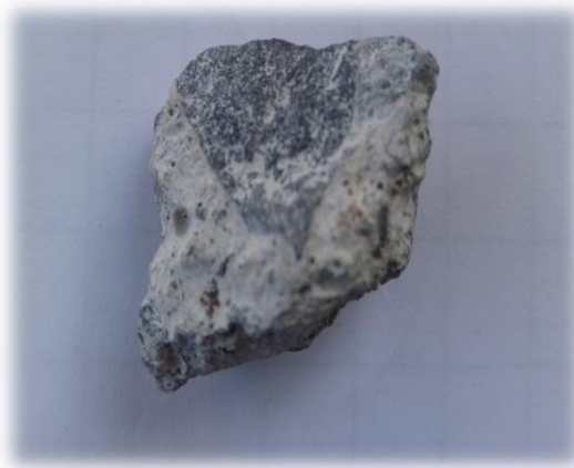
Figure 2.5: Adhered mortar on RCA (NEU Civil Engineering Laboratory, 2019)
