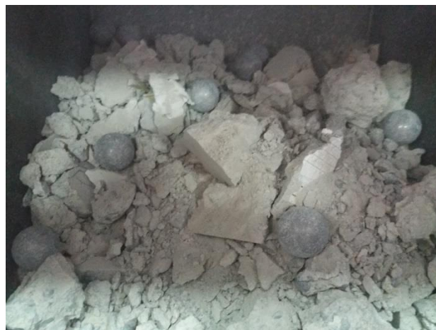
Figure 3.4: Samples crushed in Los Angeles machine with steel balls (NEU Civil Engineering Laboratory, 2019)
