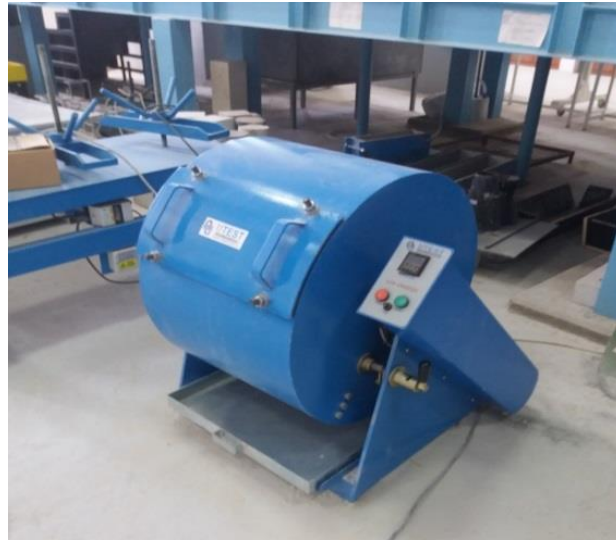
Figure 3.3: Los Angeles machine (NEU Civil Engineering Laboratory, 2019)
