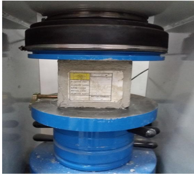
Figure 3.1: Cubes further cracking by compressive strength machine (NEU Civil Engineering Laboratory, 2019)
