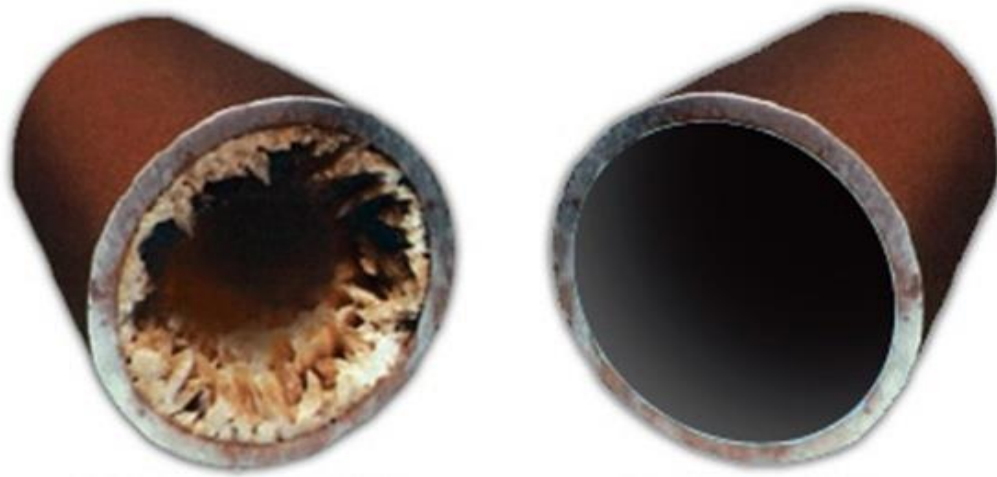
Figure 3.3: Tube with and without scale deposition (Carbtree et al., 1999)
