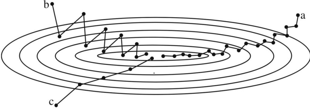
**Figure 2.3:** Effects of learning rate and momentum parameters on weight updating
