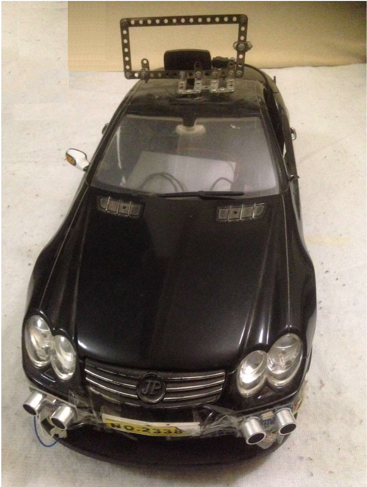
Figure 5.3: The ACC prototype-car after fitting the ultrasonic sensors
