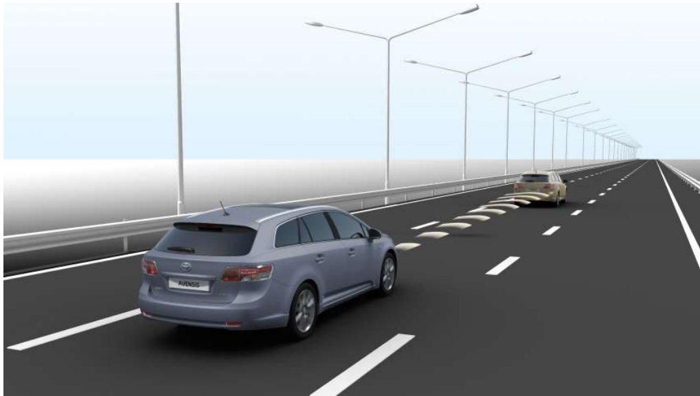
Figure 5.1: Car with ACC following another and maintaining the safe distance
