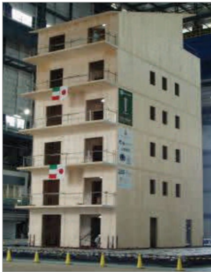
Figure 2.9: A 7-Story mass timber CLT house construction tested at the E-defence laboratory (FPInnovations, 2015)
