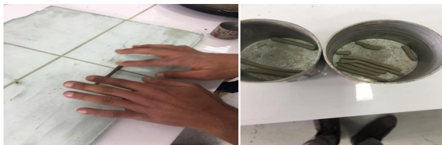
Figure 3.11: Plastic limit samples thread (a) and after dry the thread (b)
