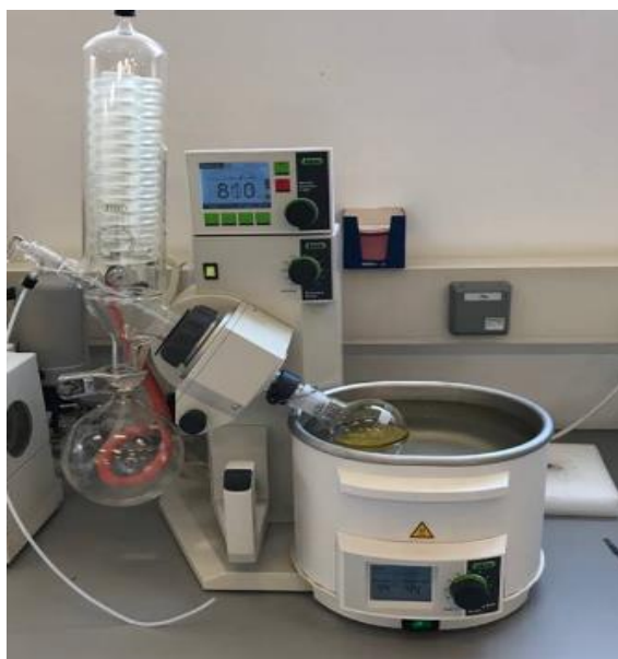
Figure 3.7: Evaporation of leaf and fruit extracts with a rotary evaporator
