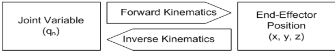
Figure 3.2: Kinematic representation of a manipulator
