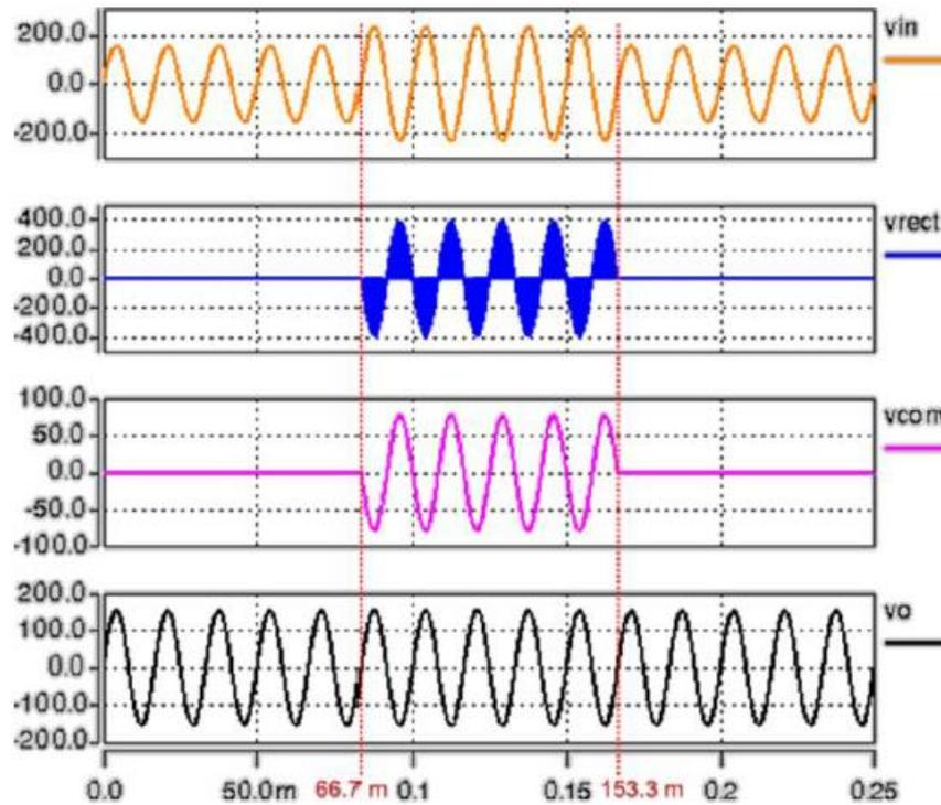
**Figure 3.13:** Simulation waveform for the DVR Buck operation for voltage swell operation
