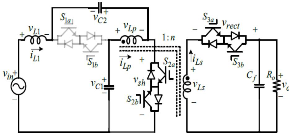
**Figure 3.4:** Boost mode equivalent circuit for  $DT$  interval
