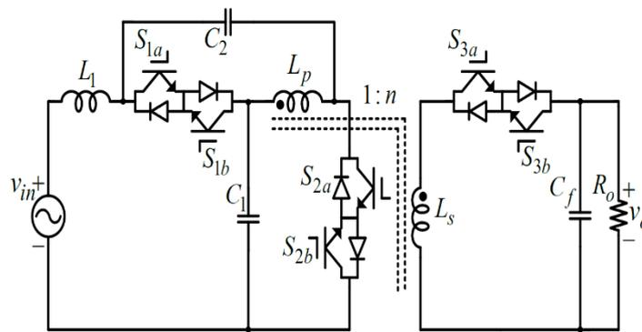
**Figure 3.1:** Ac-Ac Single-Phase HFT Isolated Z-Source Converter
