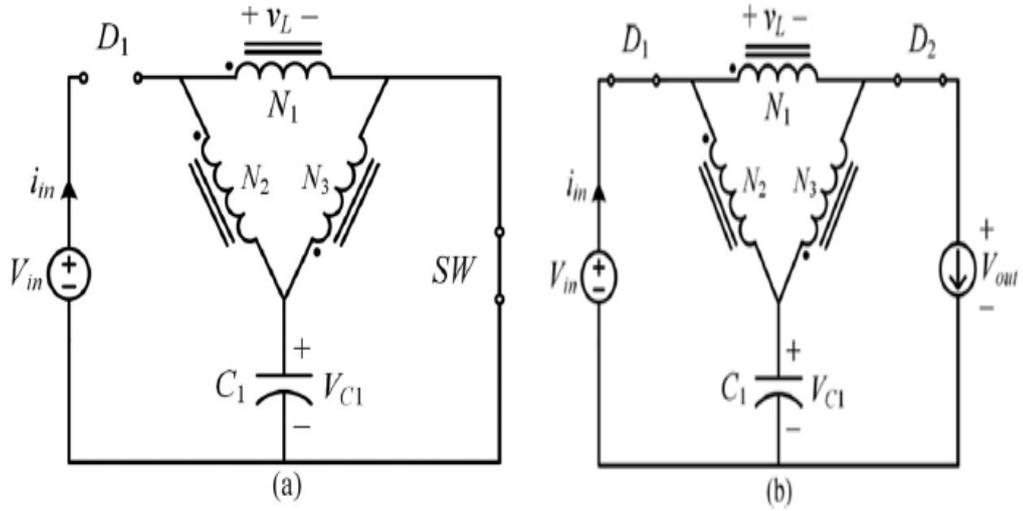
**Figure 2.9:**  $\Delta$ -Source network a) Shoot through circuit b) Non-shoot through circuit (Hakemi et al., 2017)
