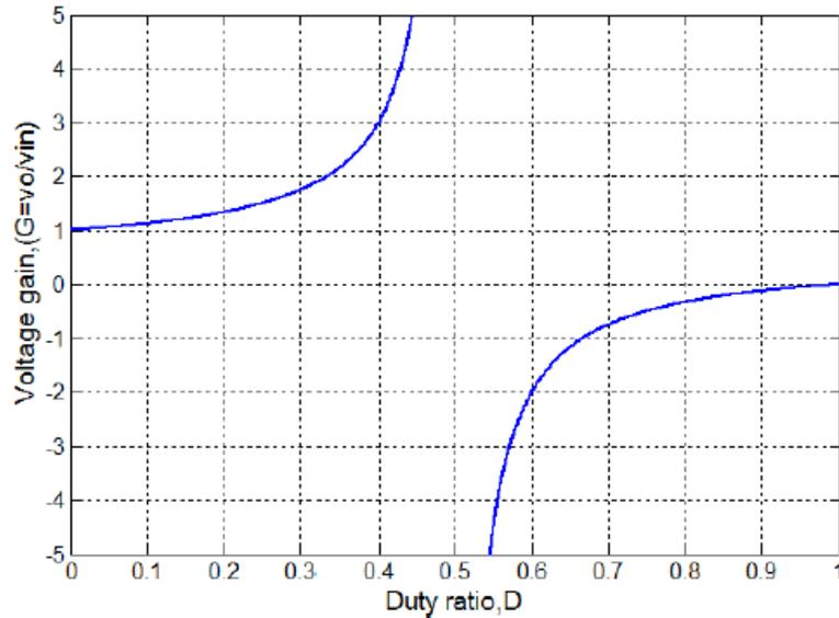
**Figure 3.10:** Plot of voltage gain against duty ratio (D) for  $n=1$  (Ahmed & Cha, 2018).
