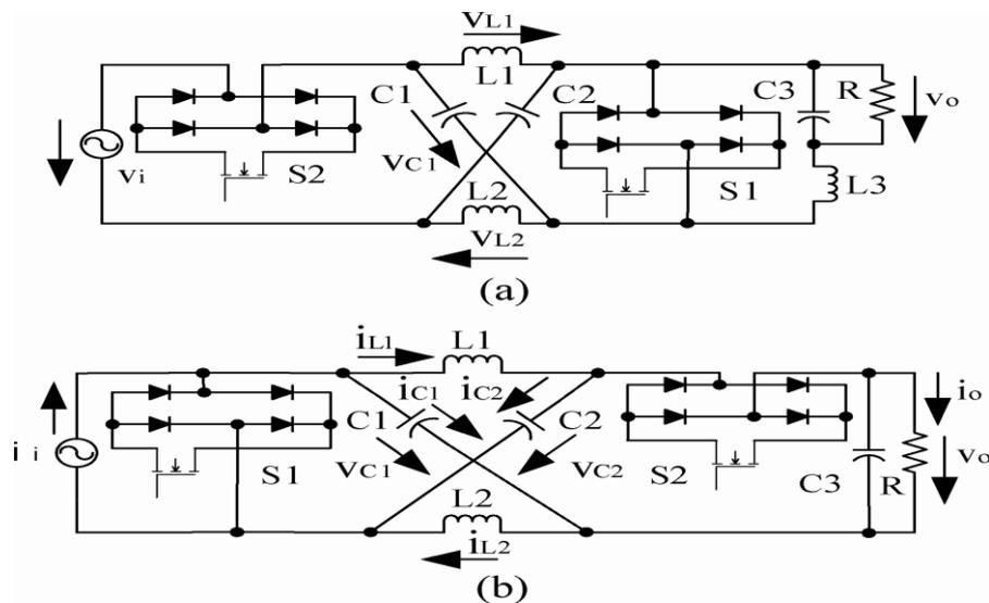
**Figure 2.13:** 1-phase Z-source ac–ac converter: (a) voltage-fed and (b) current-fed
