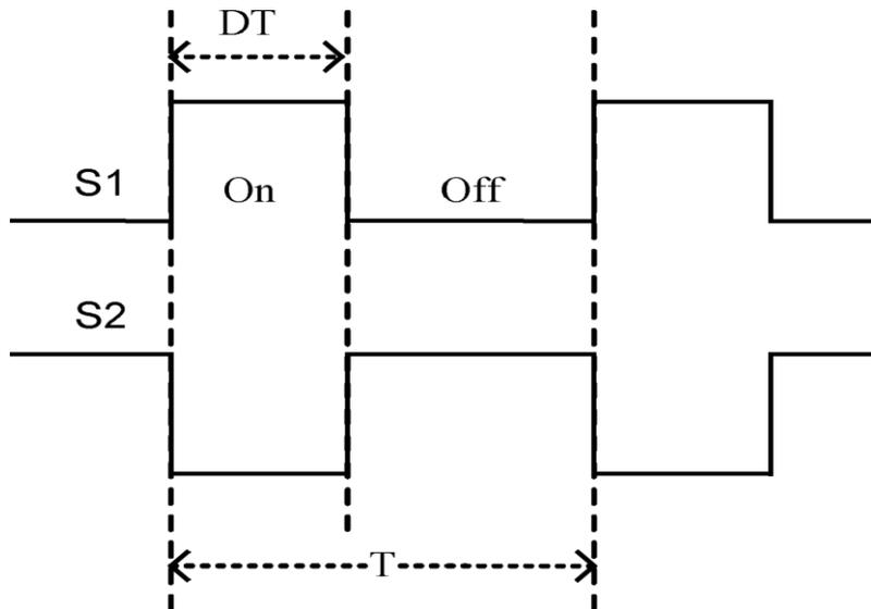
**Figure 2.14:** Duty-ratio control of Z-source ac-ac converters.
