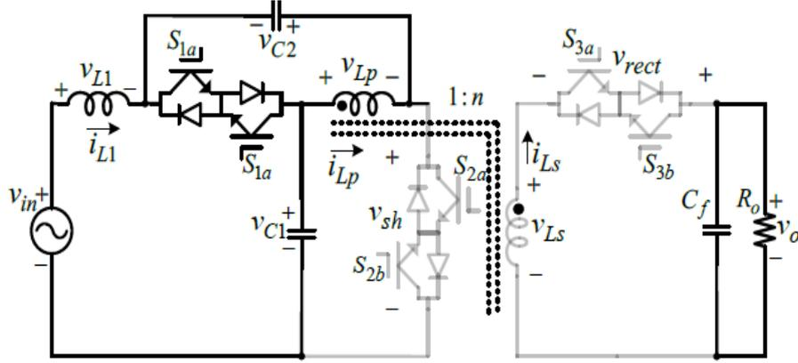
**Figure 3.6:** Boost mode equivalent circuit for  $(1-D)T$  interval
