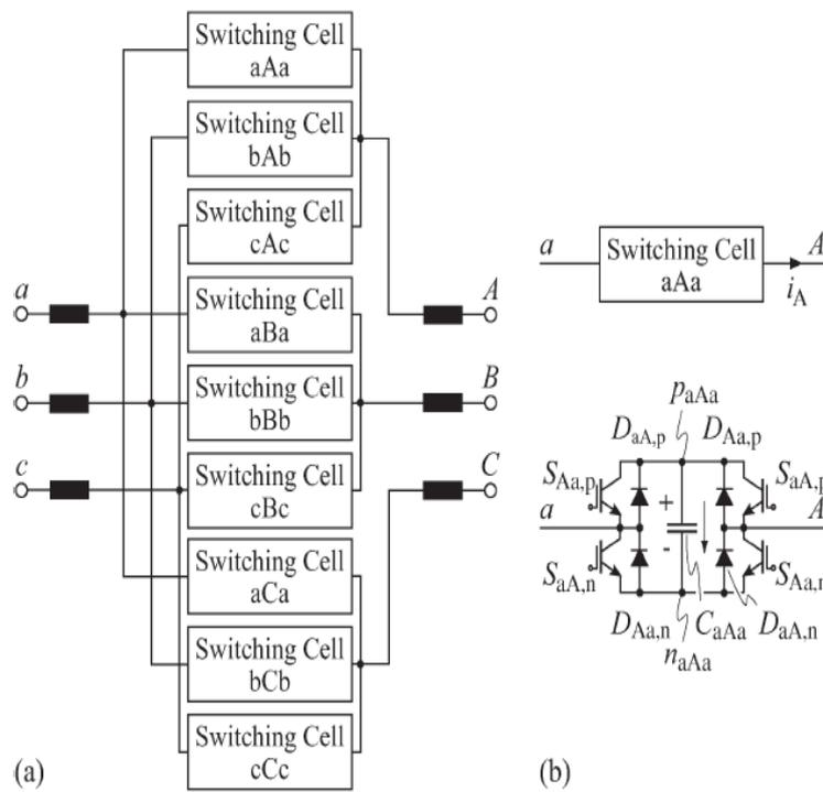
**Figure 2.6:** Hybrid matrix converters (a) Circuit topology (b) Switching cell (Erickson & Al-naseem, 2001)
