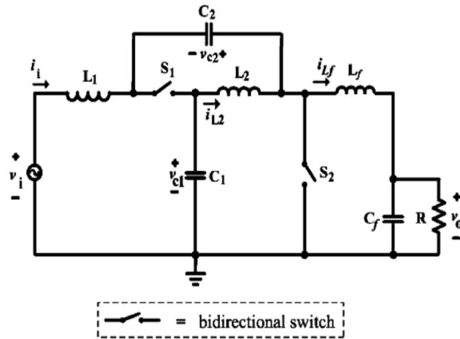
**Figure 3.2:** Single-phase Z-source ac-ac converter topology proposed in (Minh-Khai et al., 2010)
