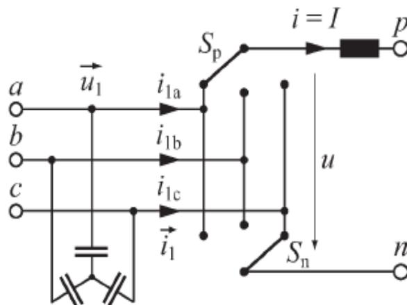
**Figure 2.4:** Current dc-link (Kuusela et al., 2000)
