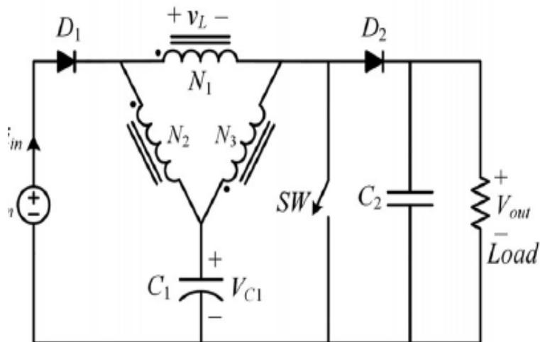
**Figure 2.8:**  $\Delta$ -Source network (Hakemi et al., 2017)
