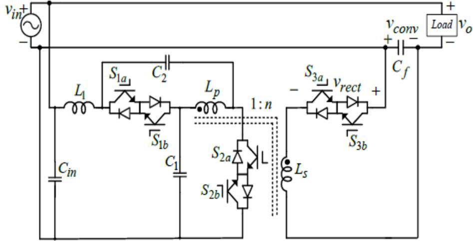
**Figure 3.11:** Application of the Converter as DVR
