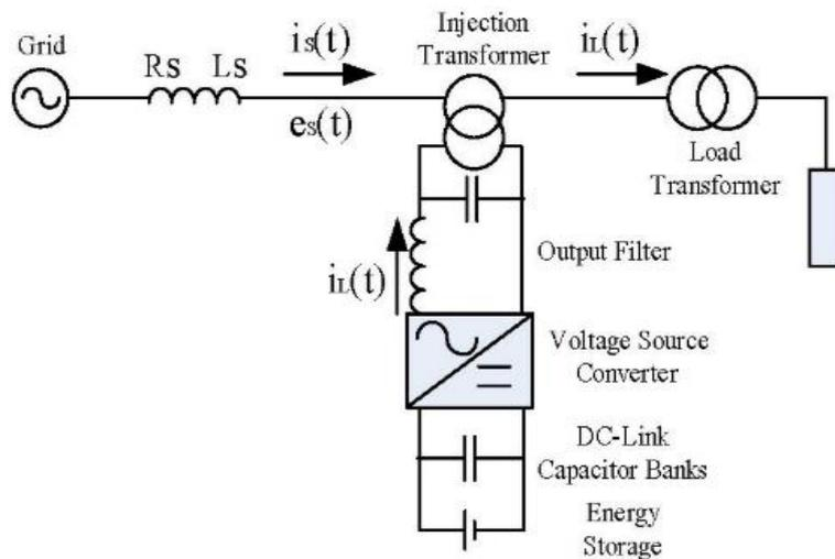
**Figure 2.17:** Typical dynamic restorer (DVR) (B. H. Li et al., 2002)
