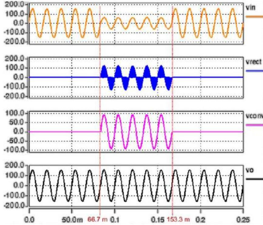
**Figure 3.12:** Simulation waveform for the DVR Boost operation for voltage sag compensation (Ahmed & Cha, 2018)
