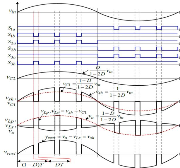
**Figure 3.3:** Boost mode key waveforms and switching pulses with soft commutation
