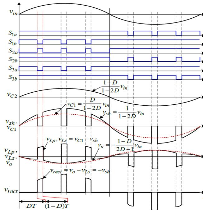
**Figure 3.7:** Buck mode key waveforms and switching pulses with safe commutation
