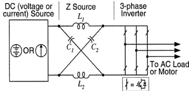
**Figure 2.7:** Basic ZSI structure (Ellabban & Abu-Rub, 2016)
