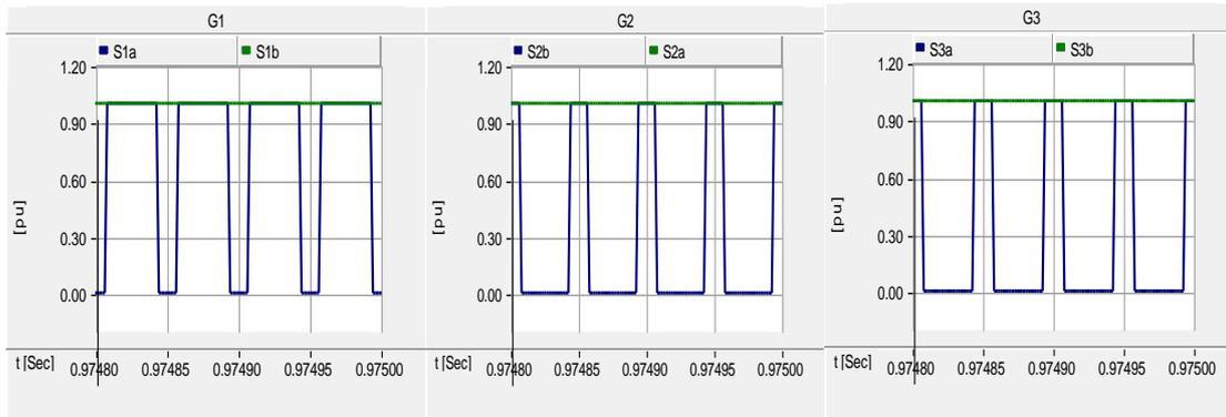
**Figure 3.19:** Triggering pulses for switches  $S_{-}(1(a,b))$ ,  $S_{-}(2(a,b))$  and  $S_{-}(3(a,b))$
