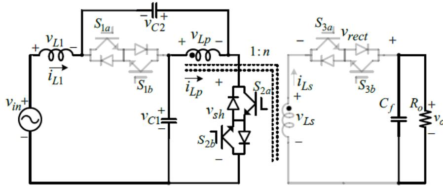
**Figure 3.9:** Buck mode equivalent circuit for  $(1-D)T$  interval (Ahmed & Cha, 2018)
