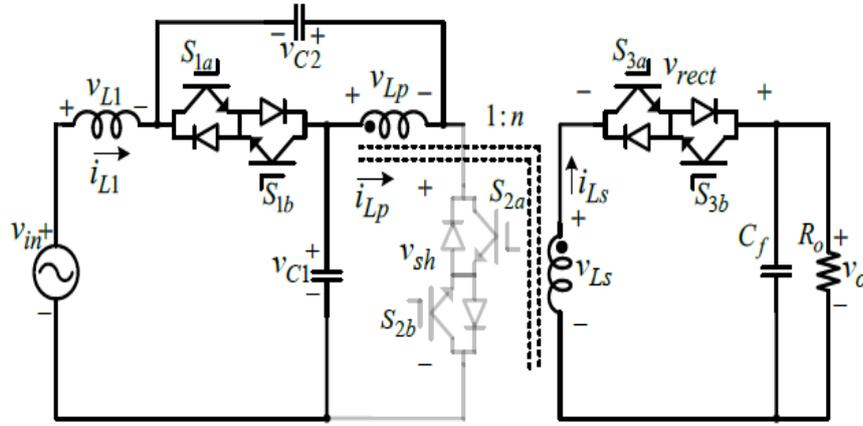
**Figure 3.8:** Buck mode equivalent circuit for  $DT$  interval
