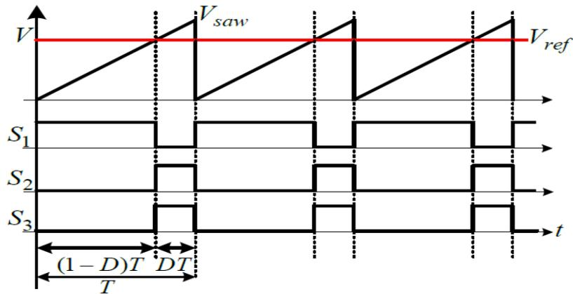
**Figure 2.16:** Pulse width modulation scheme HFTI converters (Ahmed & Cha, 2018)
