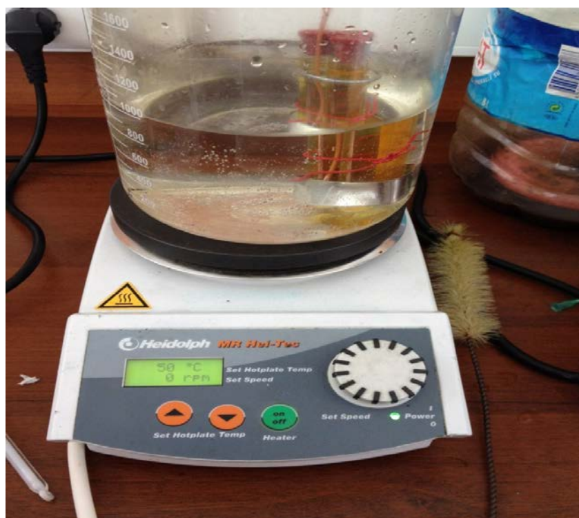
Figure 3.12: Copper strip in jojoba oil heated for three hours in a hot water bath
