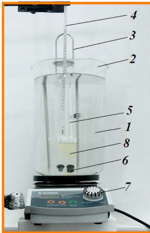
Figure 3.15: Experimental set-up for viscosity measurement
